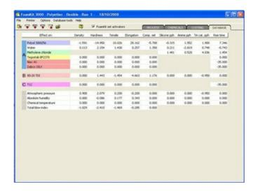
Calculations of density, hardness, other properties and process parameters are carried out by the FoamKit 3000 calculation software engine using the mathematical technique of *Logarithmic Regression*.
