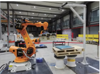
Recognition and Grasping of Condenser Tubes
