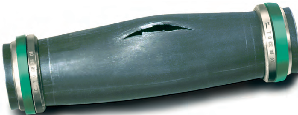
Destructive testing with 28x3 carbon steel tube. The tube burst at 1050 bars without any leakage or sweating from the sealing points.
