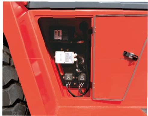
Independent integrated electric cabinet
