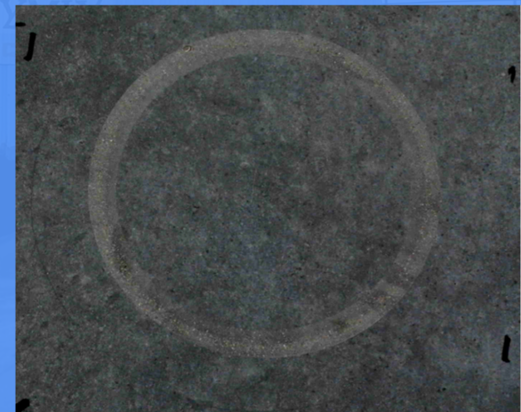
Wear ring from test 1 Mean depth 0.035 mm
