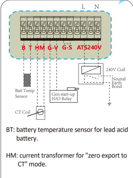
GV/GS: dry contact signal for startup the diesel generator.
