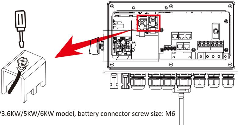
For 3KW/3.6KW/5KW/6KW model, battery connector screw size: M6
