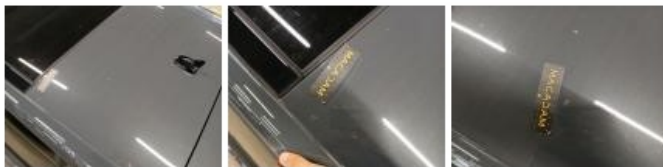
Roof, Scratch(es), Repair and paint (complete)
