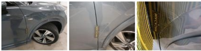
Wing trim FR, Scratch(es), Repair and paint (complete)
