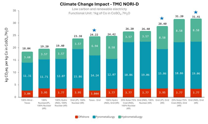
Figure E 15: Variations in climate change impact when using low carbon and renewable electricity generation sources:  $1 \log O(1) = 1 \log O(1)$ , net result.
