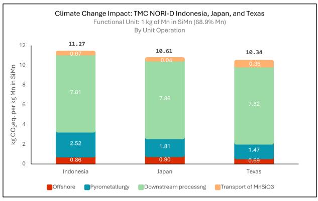
Figure 15: Climate Change Impact by Unit Operation: TMC NORI-D Indonesia, Japan, and Texas – 1 kg of Mn in SiMn
