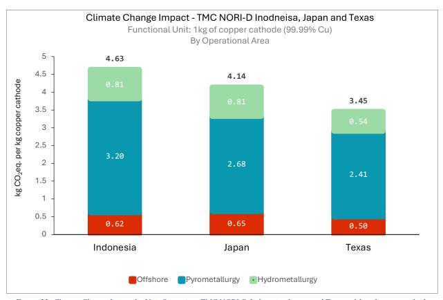
$\textit{Figure 23: Climate Change Impact by Unit Operation: TMC NORI-D Indonesia, Japan, and \textit{Texas}-1~kg~of~copper~cathode}$
