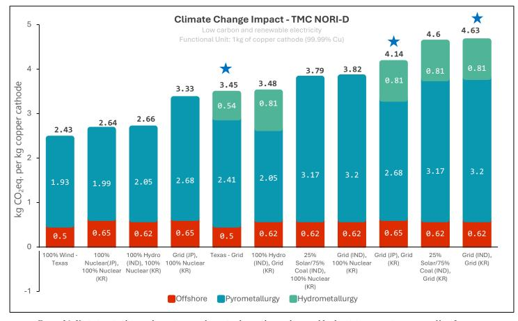
Figure 36: Variations in climate change impact when using low carbon and renewable electricity generation sources: 1kg of copper cathode.  $\Rightarrow$  = base case
