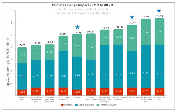
Figure 35: Variations in climate change impact when using low carbon and renewable electricity generation sources: 1kg Ni in  $NiSO_4.6H_2O$   $\star$  = base case
