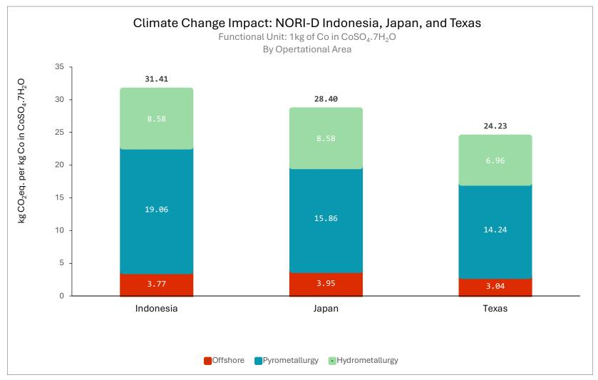
Figure E 8: Climate Change Impact by Unit Operation: TMC NORI-D Indonesia, Japan, and Texas – 1kg of Co in CoSO<sub>4</sub>.7H<sub>2</sub>O, net results.
