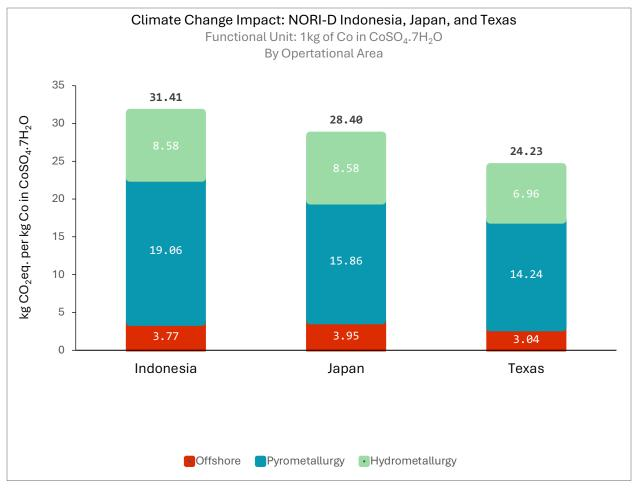
Figure 27: Climate Change Impact by Unit Operation: TMC NORI-D Indonesia, Japan, and Texas – 1 kg of Co in CoSO<sub>4</sub>.7H<sub>2</sub>O
