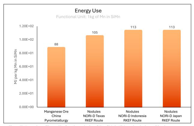
Figure 52: Comparison of Energy Use from the production of 1kg of Mn in SiMn produced using traditional manganese ores vs TMC's MnSiO<sub>3</sub>
