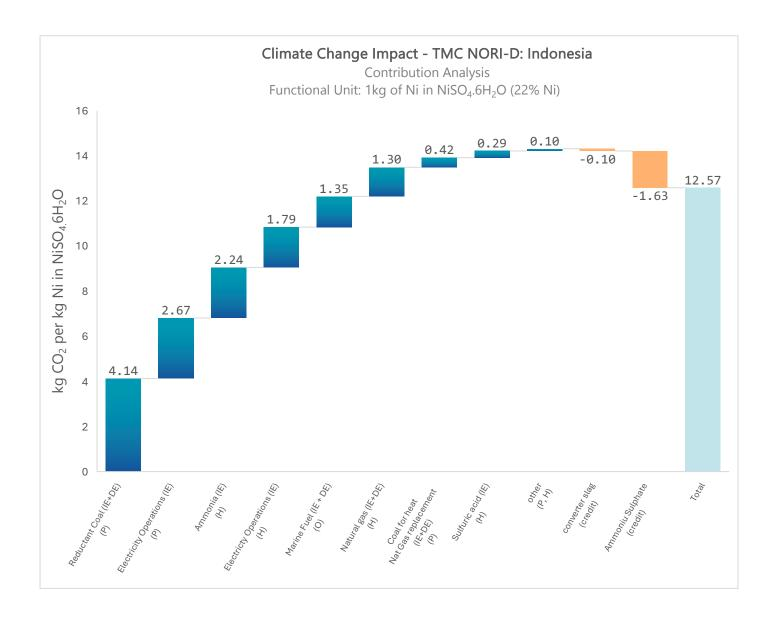
Figure 20: Climate Change Impact – Contribution Analysis: TMC NORI-D Indonesia – 1kg of Ni in NiSO<sub>4</sub>.6H<sub>2</sub>O
