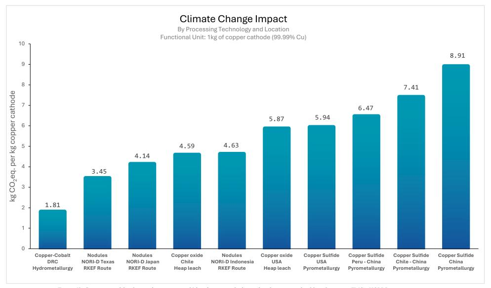
Figure 68: Comparison of the climate change impact of 1 kg of copper cathode produced via various land-based routes vs TMC's NORI-D processing routes.
