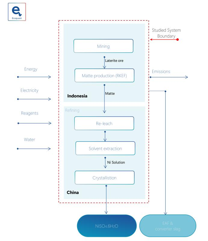
Figure 55: System Boundary for the production of NiSO<sub>4</sub>.6 $H_2O$  from saprolite ores via the Indonesia - China RKEF route.
