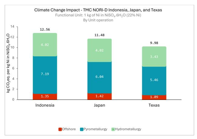
Figure 19: Climate Change Impact by Unit Operation: TMC NORI-D Indonesia, Japan, and Texas – 1 kg of Ni in NiSO4.6H<sub>2</sub>O
