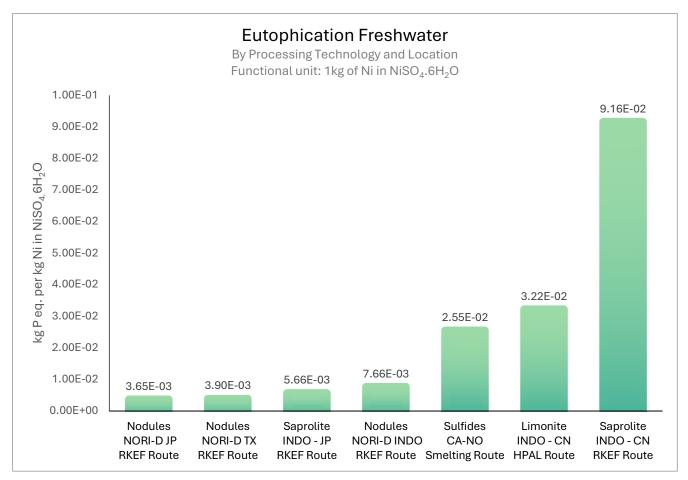
Figure 59: Comparison of the Freshwater Eutrophication Impact from the production of 1kg of Ni in NiSO<sub>4</sub>.6H<sub>2</sub>O produced using traditional land-based ores vs NORI-D Nodules.
