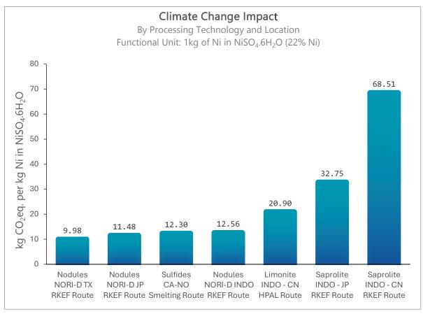
Figure 57: Comparison of the climate change impact of 1 kg of Ni in NiSO<sub>4</sub>.6H<sub>2</sub>O produced via various land-based routes vs TMC's NORI-D processing routes.
