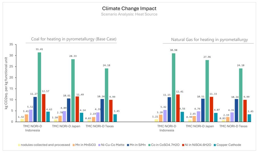
Figure 38: Scenario Analysis: Natural Gas Replacing Coal for Heat in the TMC NORI-D Indonesia and Texas Scenario
