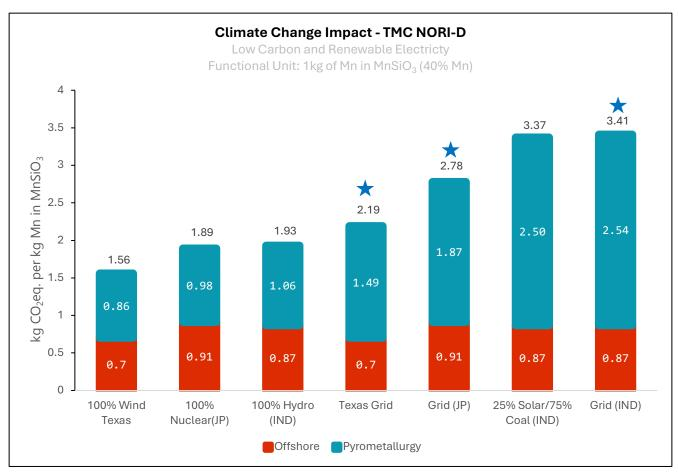
Figure 32: Variations in climate change impact when using low carbon and renewable electricity generation sources: 1kg of Mn in MnSiO<sub>3</sub>.
