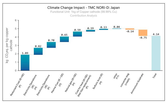
Figure 25: Climate Change Impact - Contribution Analysis: TMC NORI-D Japan - 1kg of copper cathode
