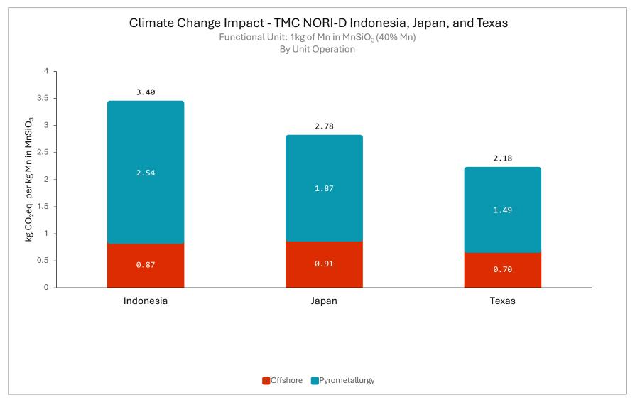
Figure E 3: Climate Change Impact by Unit Operation: TMC NORI-D Indonesia, Japan, and Texas – 1kg of Mn in MnSiO<sub>3</sub>, net results.
