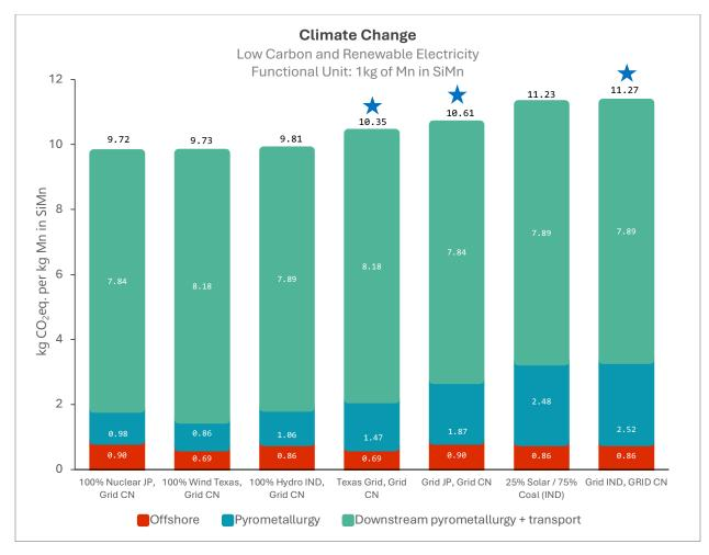
Figure 34: Variations in climate change impact when using low carbon and renewable electricity generation sources:
