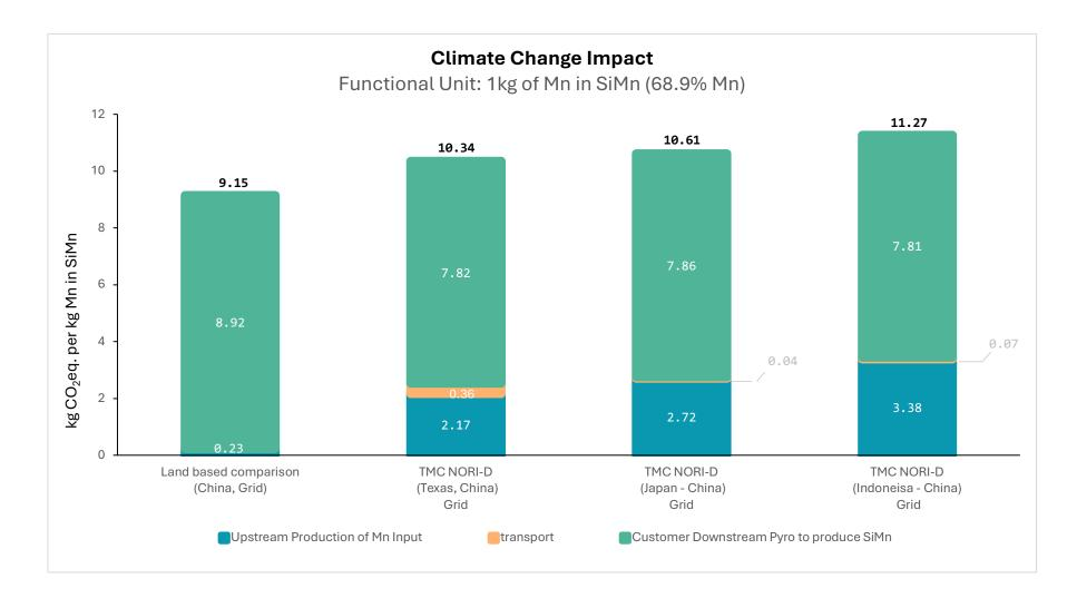
Figure E 17: Comparison of the climate change impact from the production of 1kg of Mn in SiMn produced using traditional manganese ores vs TMC's MnSiO<sub>3</sub>, net results.
