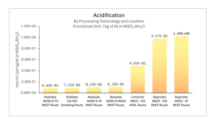
Figure 58: Comparison of the Acidification Impact from the production of 1kg of Ni in NiSO<sub>4</sub>.6H<sub>2</sub>O produced using traditional land-based ores vs NORI-D Nodules
