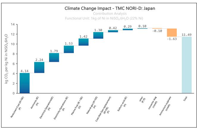
Figure 21: Climate Change Impact – Contribution Analysis: TMC NORI-D Japan – 1kg of Ni in NiSO<sub>4</sub>.6H<sub>2</sub>O
