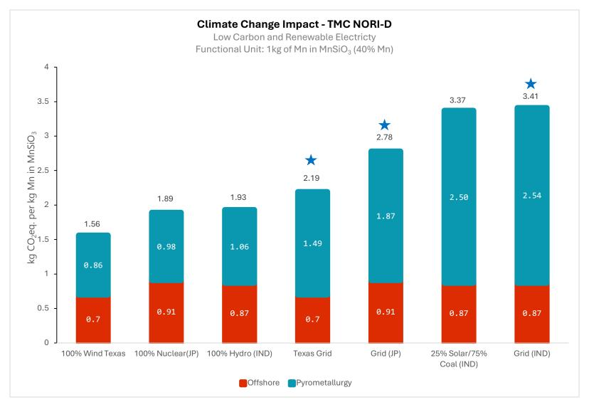
Figure E 10: Variations in climate change impact when using low carbon and renewable electricity generation sources: 1kg of Mn in MnSiO<sub>3</sub>, net results.
