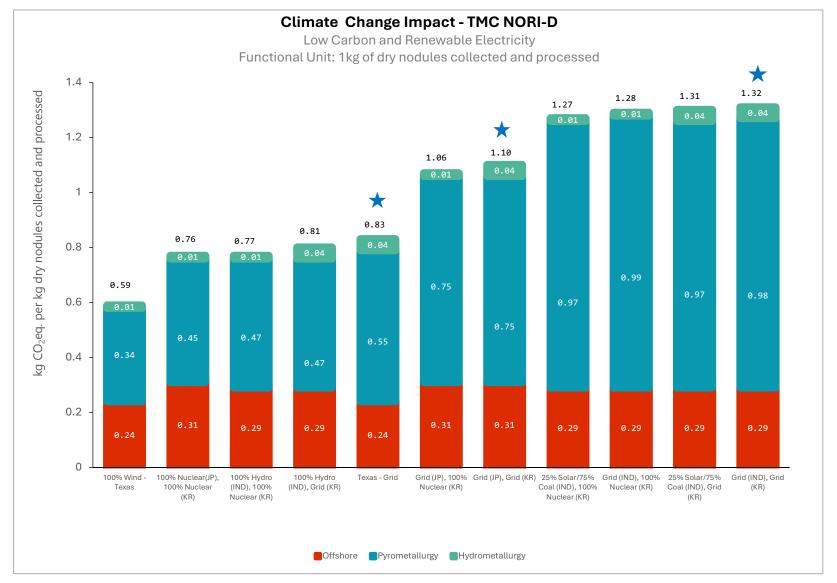
Figure E 9: Variations in climate change impact when using low carbon and renewable electricity generation sources: 1kg of dry nodules collected and processed, net results.  $\bigstar$  = base case
