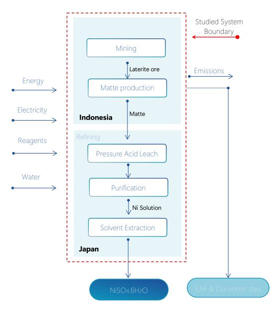
Figure 54: System Boundary for the production of NiSO4.6H2O from saprolite ores via the Indonesia - Japan RKEF route.
