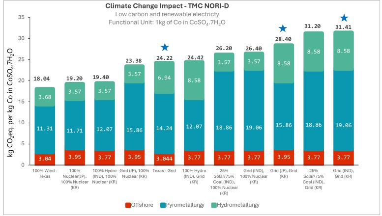
Figure 37: Variations in climate change impact when using low carbon and renewable electricity generation sources: 1kg of Co in CoSO<sub>4</sub>.7H<sub>2</sub>O.
