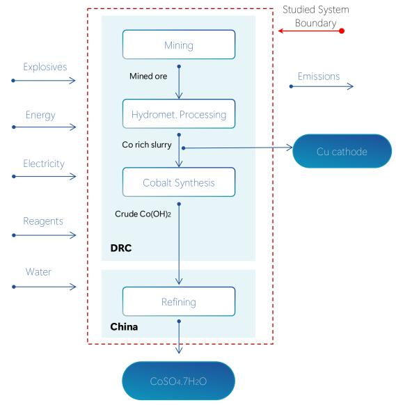
Figure 72: System Boundary for the production of CoSO<sub>4</sub>.7H<sub>2</sub>O from copper-cobalt ores via the DRC route.
