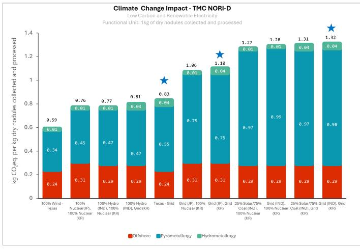
Figure 31: Variations in climate change impact when using low carbon and renewable electricity generation sources
