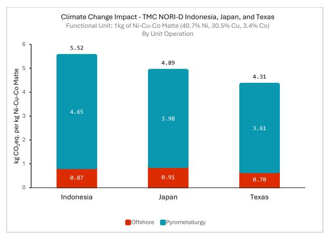
Figure 11: Climate Change Impact by Unit Operation: TMC NORI-D Indonesia, Japan, and Texas - 1 kg of Ni-Cu-Co Matte
