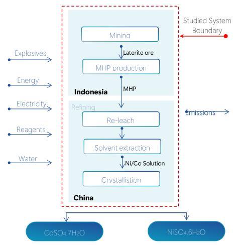
Figure 53: System Boundary for the production of NiSO<sub>4</sub>.6H<sub>2</sub>O from limonite ores via the HPAL route.
