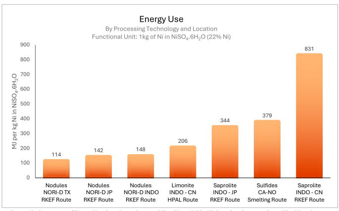
Figure 60: Comparison of Energy Use from the production of 1kg of Ni in NiSO<sub>4</sub>.6H<sub>2</sub>O produced using traditional land-based ores vs NORI-D Nodules
