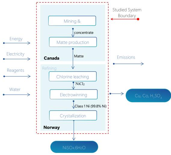
Figure 56: System Boundary for the production of NiSO<sub>4</sub>.6H<sub>2</sub>O from sulfide ores via the Canada - Norway Smelting route.
