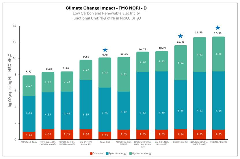
Figure E 13: Variations in climate change impact when using low carbon and renewable electricity generation sources: 1 kg of N i in  $N \text{i} SO_4.6H_2O$ , net results.  $\Rightarrow$  = base case
