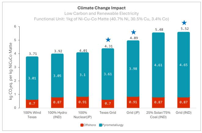
Figure 33: Variations in climate change impact when using low carbon and renewable electricity generation sources: Ikg of Ni-Cu-Co matte  $\star =$  base case
