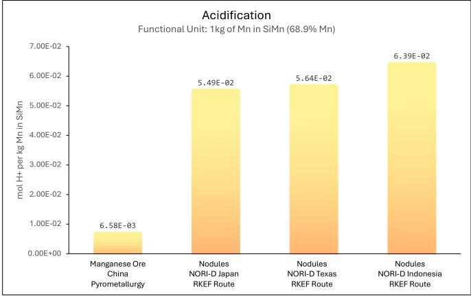
Figure 50: Comparison of the Acidification Impact from the production of 1kg of Mn in SiMn produced using traditional manganese ores vs TMC's MnSiO<sub>3</sub>
