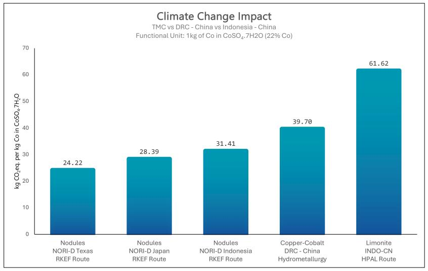
Figure E 20: Comparison of the climate change impact of 1 kg of Co in CoSO4.7H2O produced via various land-based routes vs TMC's NORI-D processing routes, net results.
