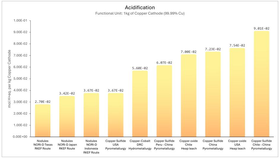
Figure 69: Comparison of the Acidification Impact from the production of 1kg of copper cathode produced via various land-based routes vs TMC's NORI-D processing routes.
