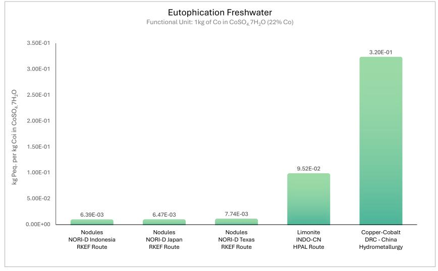
Figure 75: Comparison of the Freshwater Eutrophication Impact from the production of 1kg of Co in CoSO<sub>4</sub>.7H<sub>2</sub>O produced via various land-based routes vs TMC's NORI-D processing routes.
