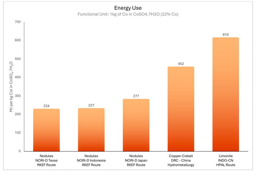
Figure 76: Comparison of Energy Use from the production of 1kg of Co in CoSO<sub>4</sub>.7H<sub>2</sub>O produced via various land-based routes vs TMC's NORI-D processing routes.
