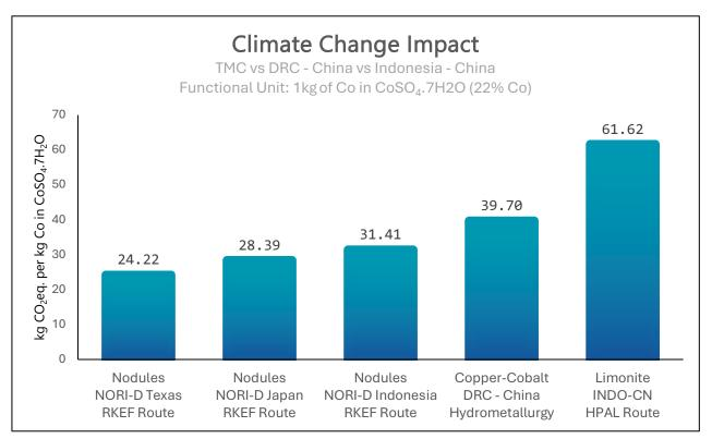
Figure 73: Comparison of the climate change impact of 1 kg of Co in CoSO<sub>4</sub>.7H<sub>2</sub>O produced via various land-based routes vs TMC's NORI-D processing routes.
