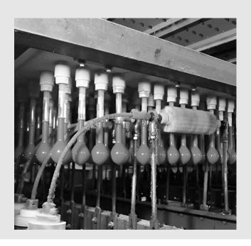
Balloon dipping machines are utilized in the production of party balloons, helium balloons, and a variety of general-purpose balloons in different shapes and sizes. Our equipment is designed to produce balloons weighing between 1.5 grams and 5 grams. We can manufacture balloons in eight distinct colors. The production capacity can reach up to 12 lakh pieces per day.
