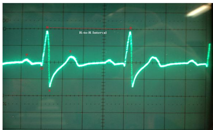
Fig. 1. Real time heart rate functioning signal (ECG) is plotted using Cathode Ray Oscilloscope (CRO)
