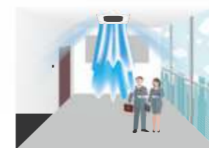
The indoor unit automatically runs when detecting human body
