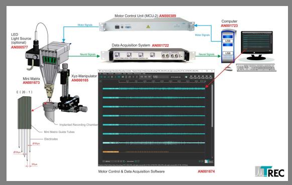
Schematic diagram of the Heptode Mini Matrix system for NHP applications with motor control unit (MCU-2) and intan data acquisition controller and graphical user interface to control the complete system .
