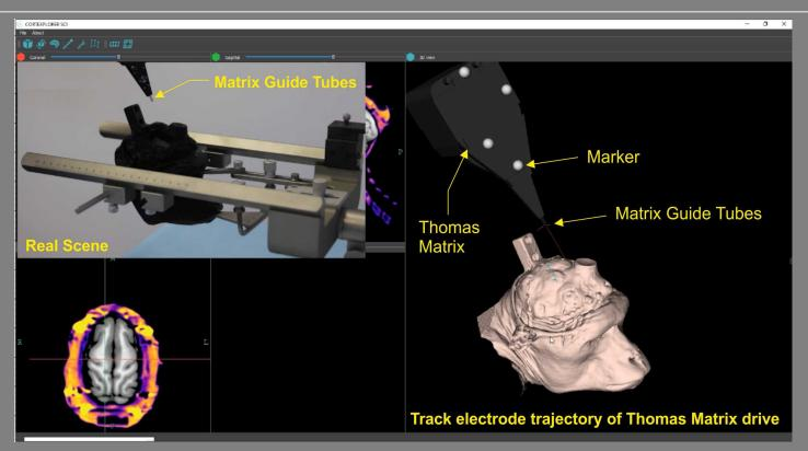
The graphical user interface of the CortExplore navigation system allows to track our Matrix microdrive by using special markers mounted the Matrix chassis surface (see picture above). The motor control unit of the Thomas Matrix microdrive sends the information about the position of each microelectrode in the brain to the CortExplore system. This enables the CortExplore navigation system software to display each electrode position on the screen in real time.
