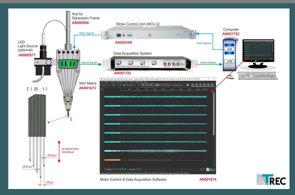
Schematic diagram of the Heptode Mini Matrix system for rodent applications with motor control unit (MCU-2) and intan data acquisition controller and graphical user interface to control the complete system .
