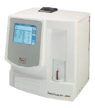
Automated cell counters sample the blood, and quantify, classify, and describe cell populations using both electrical and optical techniques.
