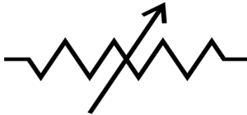
Electrical symbol of variable resistor
