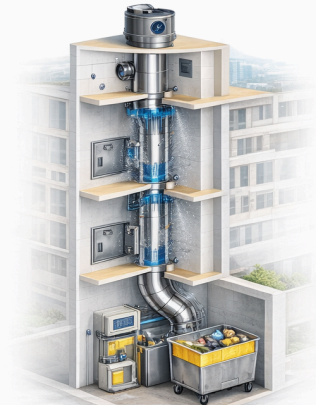
DECONTAMINATION GARBAGE CHUTE
