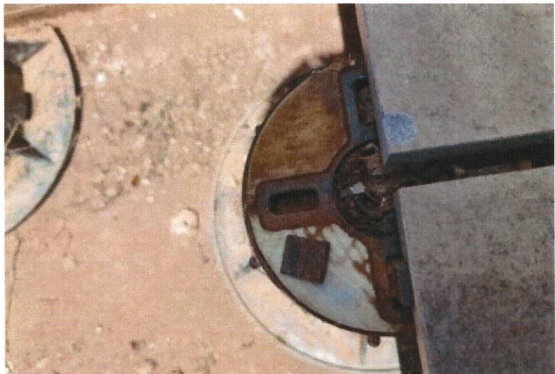
PHOTOGRAPH 9 shows broken spacer lug
