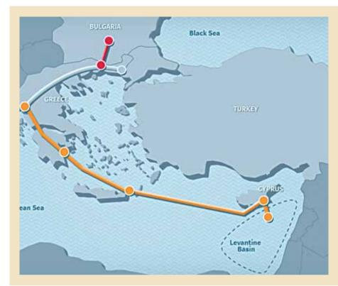
ject will be the world's longest and deepest sub-sea pipeline, with the capacity to transport 10 billion cubic metres of gas per year, a total cost of around €5 billion, with an initial €70 million coming from the EU as part of its pre-FEED studies. Although technically the project is very challenging due to the deep sea, the financial support is already in place, so the pipeline could theoretically be completed by 2025, with the eventual aim of helping secure Europe's energy future.
