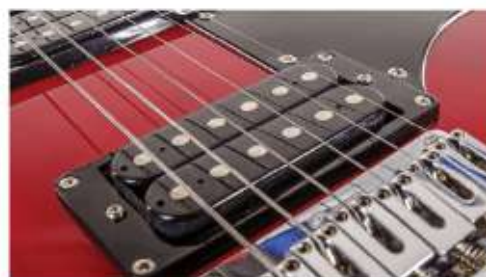
Figure 21.1 An electric guitar pickup, which comprises six permanent magnets and coils of wire around a bobbin
