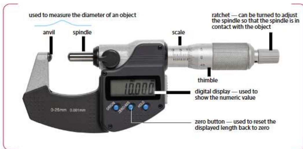
Figure 1.7 Parts of the digital micrometer screw gauge and their uses
