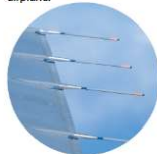
Figure 15.24 Static discharge rods on the wing of an airplane.
