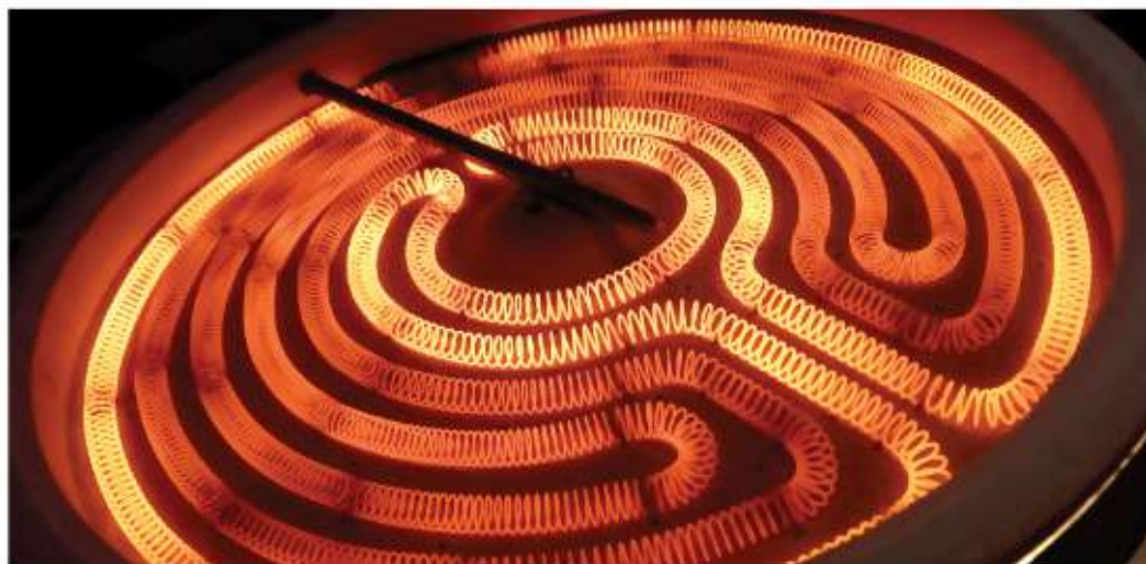
Figure 18.1 Heating elements are usually made from long and thin nichrome or iron-chromium-aluminium wires that are wound into long cylindrical shapes to increase the length of the wires used.
