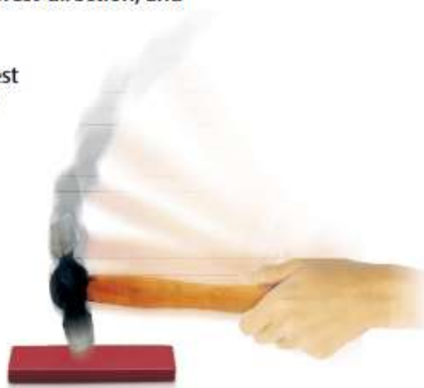
Figure 19.13 Hammering the magnet placed in the east-west direction can cause it to lose its magnetism.
