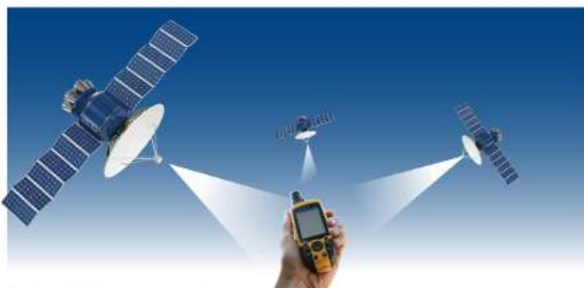
Figure 13.8 Microwave signals received from at least three GPS satellites allow a receiving device such as a GPS device or a mobile phone to work out its location.
