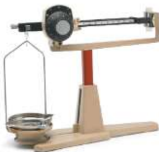
Figure 3.7 A beam balance is used to measure mass.
