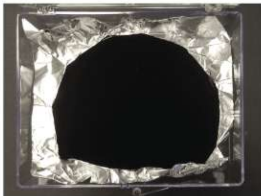
Figure 14.3 An aluminium foil with a part coated with Vantablack, which is one of the darkest substances known.
