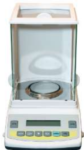
Figure 3.6 The electronic balance is a commonly used weighing instrument for measuring mass. In fact, electronic balances measure weight, but they are calibrated to give readings for mass.
