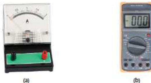
Figure 16.4 Both the (a) analogue ammeter and (b) a digital multimeter are used in measuring electric current.
