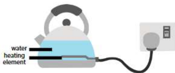
Figure 7.27 Energy is transferred electrically from the power source to the internal stores of the heating element and water.
