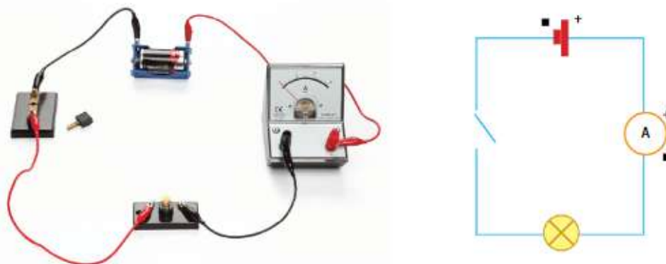
Figure 17.1 (a) An actual electric circuit and (b) its equivalent circuit diagram
