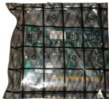
Figure 15.28 Electronics protected by an anti-static bag
