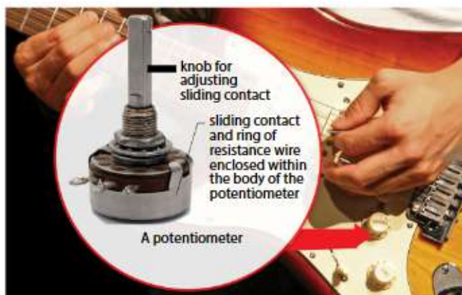
Figure 17.20 Potentiometers are used in electric guitars to control the volume.
