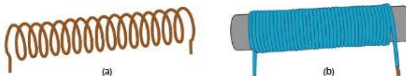
Figure 20.7 Solenoid (a) without soft iron core (b) with soft iron core
