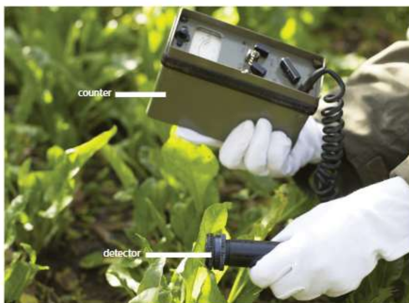
Figure 22.8 A GM counter is used to measure ionising nuclear radiation.
