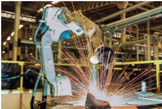
▲ Figure 6.12 Robot welder
