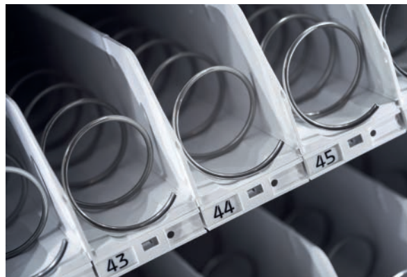
▲ Figure 3.12 Helix used in a typical vending machine
