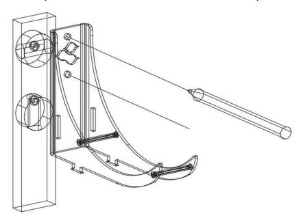
3. Insert the wall plugs into the drilled holes.
