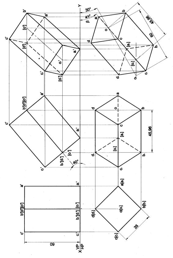
**Problem 4** A square prism 35 mm sides of base and 60 mm axis length rests on HP on one of its edges of the base. Draw the projections of the prism when the axis is inclined to HP at 45° and VP at 30°. **Solution**
