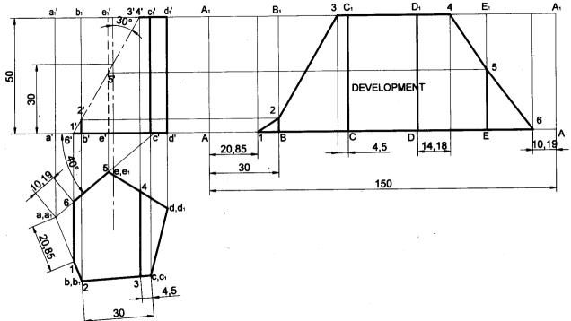
**Problem 13** A pentagonal prism of base sides 30mm and axis length 60mm rests with its base on HP and an edge of the base inclined at 45° to VP. It is cut by a plane perpendicular to VP, inclined at 40° to HP and passing through a point on the axis, at a distance of 30 mm from the base. Develop the remaining surfaces of the truncated prism. **Solution**
