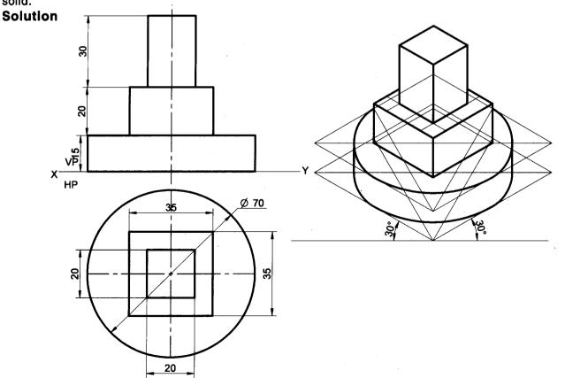
**Problem 31** Following figure shows the front and top views of solid. Draw the Isometric projection of the solid. **Solution**
