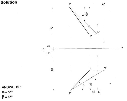
**Problem 20** A point P is 40 mm above HP and 20 mm infront of VP another point Q is 20 mm above HP and 50 mm infront of VP. The top view of line PQ is inclined at 30° to XY. Draw the projections. **Solution**
