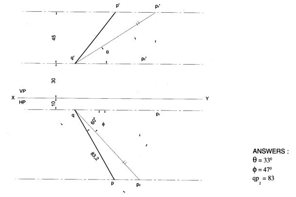
**Problem 6** A line PQ 85 mm long has its end P 10 mm above the HP and 15 mm infront of the VP. The top view and front view of line PQ are 75 mm and 80 mm respectively. Draw its projections. Also determine the true and apparent inclinations of the line.
