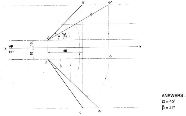
Problem 39 Two lines AB and AC make an angle of 120° between them in their front view and top view. AB is parallel to both the HP and the VP. Determine the real angle between AB and AC. Solution
