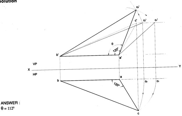
Problem 40 The elevation of a line AB 90 mm long, is inclined at 30° to HP and measures 70 mm. The end A is 20 mm above HP and is in VP. Draw the projections of the line and find its inclination with VP. Solution
