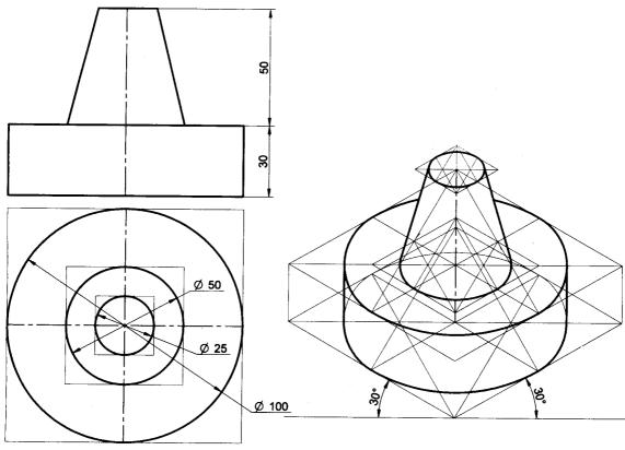
**Problem 23** A frustum of cone base diameter 50mm, top diameter 25mm and height 50mm is placed centrally on a square slab side-80mm and thickness-30mm. Draw the isometric projection of the combination. **Solution**
