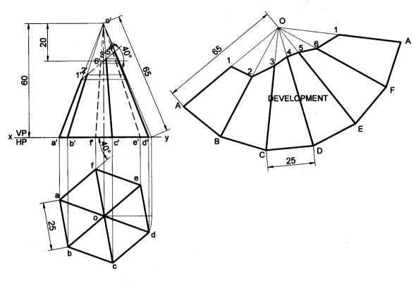
Problem 28 A hexagonal pyramid of sides 35mm and altitude 65mm is resting on HP on its base with two of the base sides perpendicular to VP. The pyramid is cut by a plane inclined at 30° to HP and perpendicular to VP and is intersecting the axis at 30mm above the base. Draw the development of the remaining portion of the pyramid. Solution
