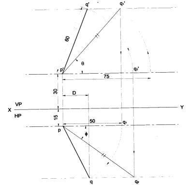
**ANSWERS** :  $\theta = 48^{\circ}$  $\phi = 37^{\circ}$ D = 22 **Problem 43** A straight line AB measuring 80 mm long has the end A in the HP and 25 mm infront of the VP. Its mid point M is 25 mm above HP and 40 mm infront of the VP. Draw the views of the line and determine the inclination of the line with HP and VP and also find distance between end projectors.
