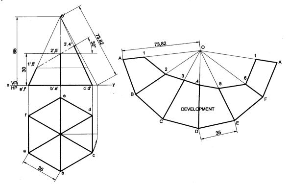
**Problem 29** A hexagonal pyramid 25 mm side of base and axis 65 mm long is resting on its base on HP with one of the edges of the base parallel to VP. It is cut by a vertical section plane at a distance of 8 mm from the axis towards right side. Develop the lateral surface of the left part of the pyramid. **Solution**
