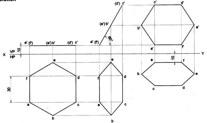
**Problem 34** A regular hexagonal lamina of sides 30mm is lying in such a way that one of its sides touches both the reference planes. If the lamina makes 60° with HP, draw the projections of the lamina. **Solution**
