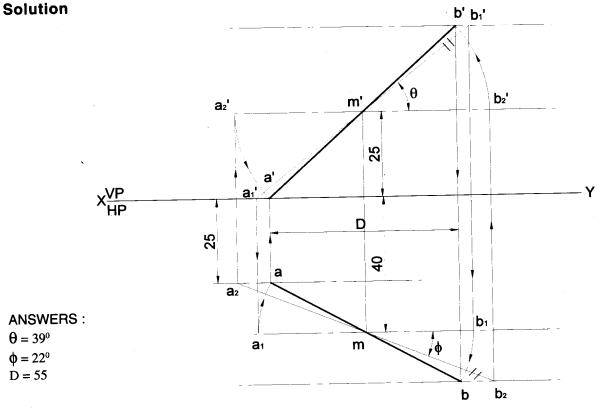
**Problem 44** The end A of a line AB is in HP and 25mm in front of VP. The end B is 25 mm infront of VP and 50mm above HP. The distance between the end projectors when measured parallel to the line of intersection of HP & VP is 65mm. Draw the projections of the line AB and determine its true length and true inclinations with HP & VP. **Solution**
