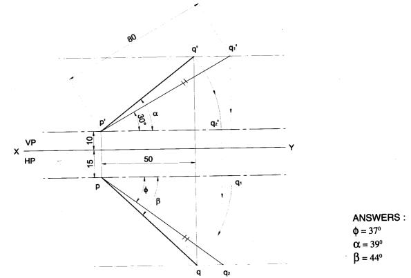
**Problem 42** The top view of a line PQ 75 mm long measures 50 mm and the front view measures 60 mm. The end P is 30 mm above HP and 15 mm infont of VP. Draw the projections of the line and find its true inclinations with HP and VP. Find length of front view and distance between the end projectors.
