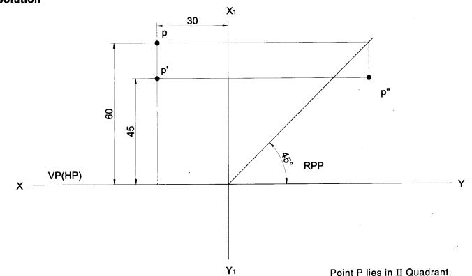
**Problem 17** Draw all the three views of a point P lying 60 mm below HP, 70 mm in front of VP and 40 mm from the RPP. Also state the quadrant in which it lies. **Solution**
