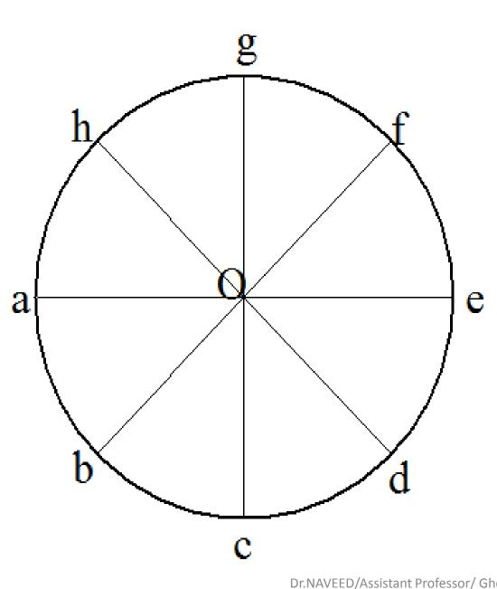
1. Construct circle by circle by center point command. 2. Draw a line oe 3. Select the line oe 4. Click on Circular Pattern command. e 5. Type No. of Count = 8 and Angle = 3606.Click at center point O and then click on Finish button.
