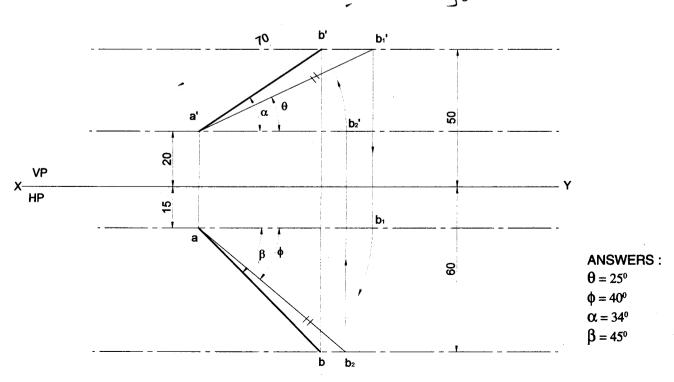
**Problem 11** The front view of a 90 mm long line which is inclined at 45° to the XY line, measures 65 mm. End A is 15 mm above the XY line and is in VP. Draw the projections of the line and find is inclinations with HP and VP. **Solution**
