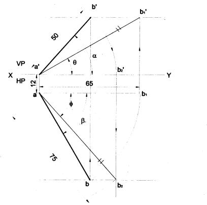
**Problem 18** A line AB, 65 mm long, has its end A 20 mm above the H.P and 25 mm in front of the V.P The end B is 40 mm above the H.P. and 65 mm in front of the V.P. Draw the projections of AB and show its inclinations with the H.P. and the V.P.
