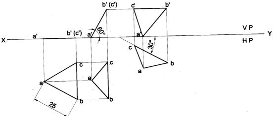
**Problem 5** A triangular plane lamina of sides 25mm is resting on HP with one of its corners touching it, such that the side opposite to the corner on which it rests is 15mm above HP and makes an angle of 30° with VP. Draw the top and front views in this position. Also determine the inclination of the lamina to the reference plane. **Solution**
