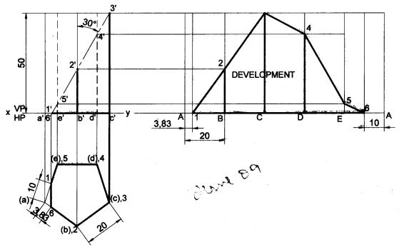
**Problem 11** A regular pentagonal prism of height 60mm and base edge 30mm rests with its base on HP. The vertical face closest to VP is 30° to it. Draw the development of the truncated prism with its truncated surface inclined at 60° to its axis and bisecting it.
