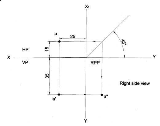
**Problem 48** A point P is 15 mm above HP & 25 mm in front of VP. Another point Q is 25 mm behind VP and 40 mm below HP. Draw their projections when the distance between their projectors parallel to XY line is zero mm. Add the right side view only to point Q. **Solution**
