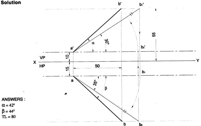
**Problem 8** The top view of a line 75 mm long measures 50 mm. the end P is 30 mm infront of VP and 15 mm above HP. The end Q is 15 mm infront of VP and above HP. Draw the projections of the line and find its true inclinations with HP and VP.
