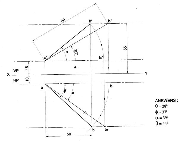
**Problem 46** The end A of a line AB is in HP and 25mm in front of VP. The end B is 10 mm in front of VP and 50mm above HP. The distance between the end projectors when measured parallel to the line of intersection of HP & VP is 80 mm. Draw the projections of the line AB and determine its true length and true inclinations with HP & VP. **Solution**
