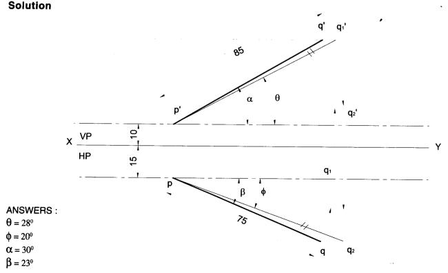
**Problem 7** A line has its end A 10 mm above HP and 15 mm infront of VP. The end B is 55 mm above HP and line is inclined at  $30^{\circ}$  to HP and  $35^{\circ}$  to VP. The distance between the end projectors is 50 mm. draw the projections of the line. Determine the true length of the line and its inclination with VP.
