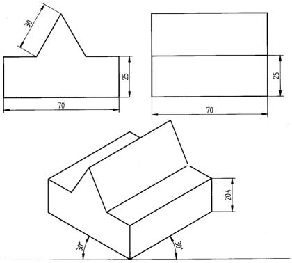
**Problem 45** A square prism of base side-30mm and length-70mm, is resting on its rectangular face on top of a square slab side -70mm and 25mm-thick. Draw the isometric projection of the combination **Solution**
