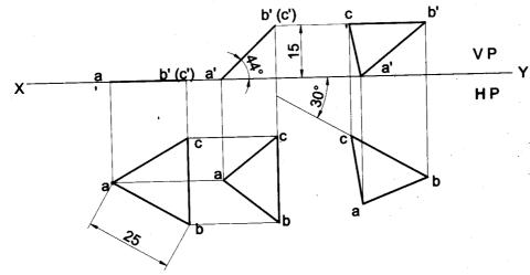
**Problem 6** A 30°-60° setsquare of 60mm longest side is so kept such that the longest side is in HP, making an angle of 30° with VP. The set square itself is inclined at 45° to HP. Draw the projections of the setsquare. **Solution**
