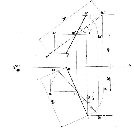
**Problem 36** A straight line PQ is inclined at 45° to HP and 30° to VP. The point P is in HP and the point Q is in VP. The length of the straight line is 65 mm. draw the projections of the straight line AB. Solution
