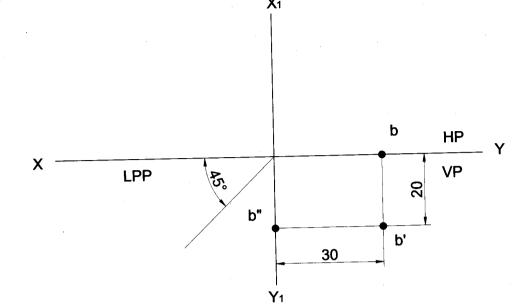
**Problem 24** A point A is 20 mm above HP & 25 mm in front of VP. Another point B is 25 mm behind VP and 40 mm below HP. Draw their projections when the distance between their projectors parallel to XY line is zero mm. Add the right side view only to point B.
