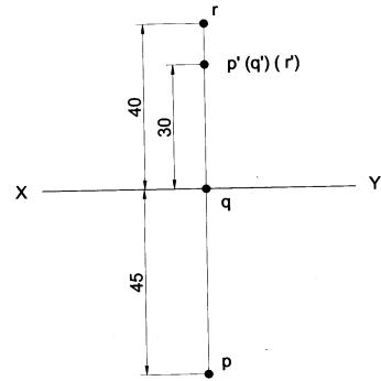
P - I Quadrant Q - I as well as II Quadrant R - II Quadrant **Problem 29** A point 'M' is 30 mm in front of VP and 20 mm above HP. another point N in 15 mm behind VP & 25mm below HP. The horizontal distance between the points parallel to XY line is 50 mm. Draw the projections of the points M & N and Join their front and top views. Draw the right side view for the point N only. **Solution**
