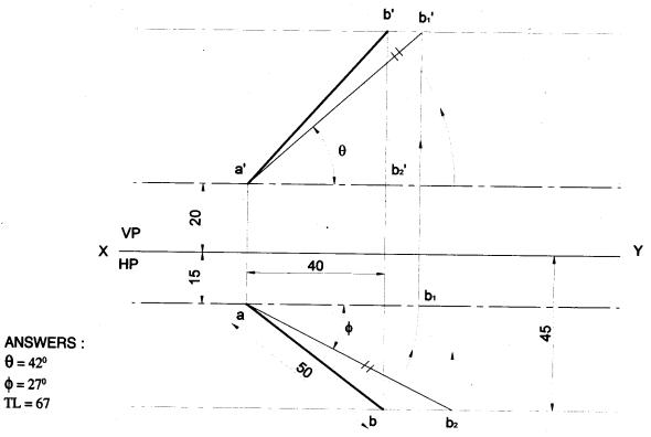
**Problem 14** The point B of a line AB is on the horizontal plane, the top view of the line makes an angle of 30° with XY line, being 80 mm. The point A is on the vertical plane and 50 mm above the horizontal plane. Draw the top and front views of the line and obtain the true length of the line. Also find the inclinations of the line with the two planes. Solution
