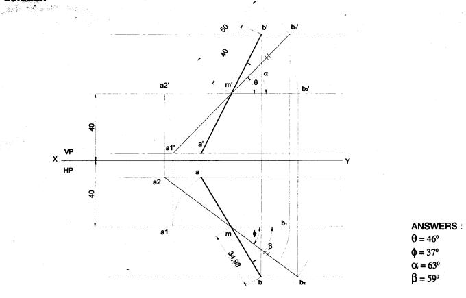
Problem 23 A line has its end A 15 mm above HP and 10 mm infront of VP. The end B is 55mm above HP and the line is inclined at 30° to HP. The distance between the end projectors is 50 mm. draw the projections of the line and determine the true length of the line and its inclinations with VP.
