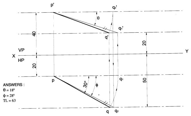
**Problem 21** The top view of a line PQ is 70 mm and front view is 60 mm long. The end Q is nearer to both HP and VP than the end P and is 15 above HP and 20 mm infront of VP. Draw the projections of the line if the distance between projectors is 50 mm. **Solution**
