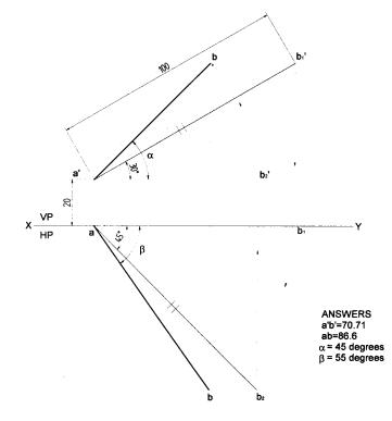
**Problem 31** Draw the projections of a line PQ and find its true length and inclinations when the line is inclined at  $30^{0}$  to the HP and  $45^{0}$  to the VP. The line is having one of its ends 15 mm above HP and 20 mm in front of VP. The distance between the end projectors on the XY line is 60 mm.
