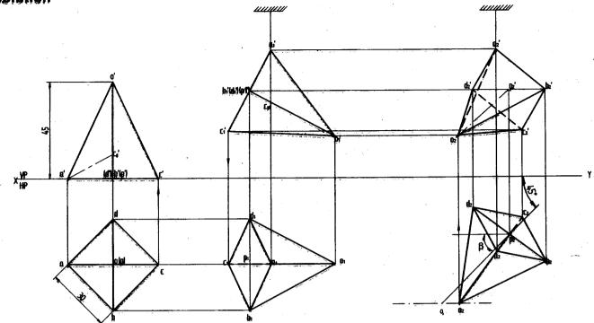
**Preblem 50** A sone of base dia. 40 mm and axis length 50 mm is resting on HP on a point on the circumference of its base such that its apex is at 40 mm above the HP and its top view of the axis is inclined at 60° to VP. Draw the top and front views of the solid. Also, determine the inclinations of the axis when the base is nearer to the observer.
