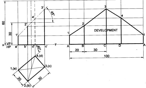
**Problem 9** A rectangular prism of base size 25mmx40mm and axis length 65mm is resting on HP on ite base with the longer side of base inclined at 30° to VP. It is cut by a plane inclined at 40° to HP and perpendicular to VP and passes through the extreme left corner of base. Draw the development of the lateral surface of the remaining portion of the prism.
