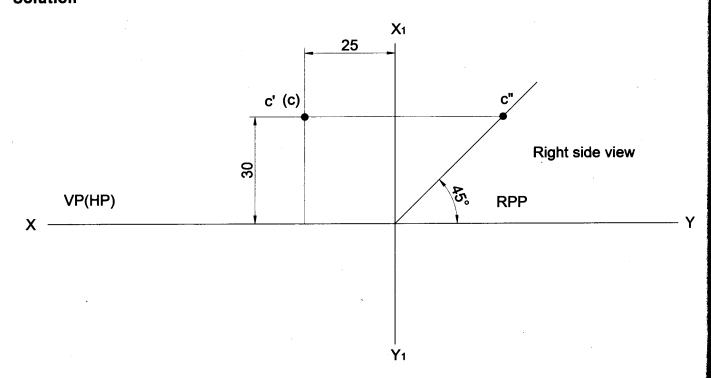
**Problem 45** A point is lying on VP, 10 mm below HP & 30 mm behind / in front / from LPP. Draw its projections and name the side view. **Solution**
