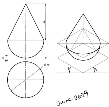
**Problem 27** Following figure shows the front and side views of solid. Draw the Isometric projection of the solid.
