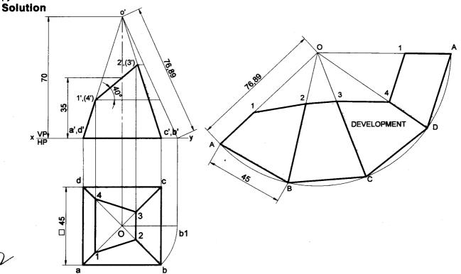
**Problem 19** A square pyramid base 40mm side and axis 65mm long has its base on HP and all the edges of the base are equally inclined to VP. It is cut to with an inclined section plane so as the truncated surface at 45° to its axis, bisecting it. Draw the development of the truncated pyramid. **Solution**
