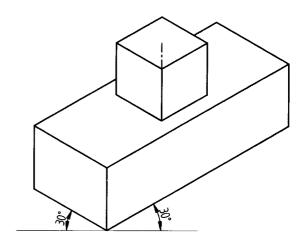
**Problem 42** Two rectangular plates are placed centrally with dimensions (lxbxh)100mmx60mmx20mm and 100mmx40mmx20mm such that longer edges are parallel. Draw the isometric projection of the combination **Solution**
