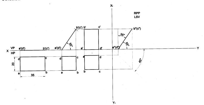
**Problem 14** A rectangular lamina of 35mm x 20mm rests on HP on one of its shorter edges. The lamina is rotated about the edge on which it rests till it appears as a square in the top view. The edge on which the lamina rests is inclined 30° to VP. Draw its projections and find its inclination to HP. **Solution**
