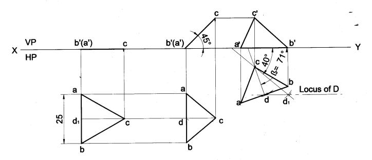
**Problem 3** A triangular lamina of 25mm sides rests on one of its corners on VP such that the median passing through the corner on which it rests is inclined at 30° to HP and 45° to VP. Draw its projections. **Solution**
