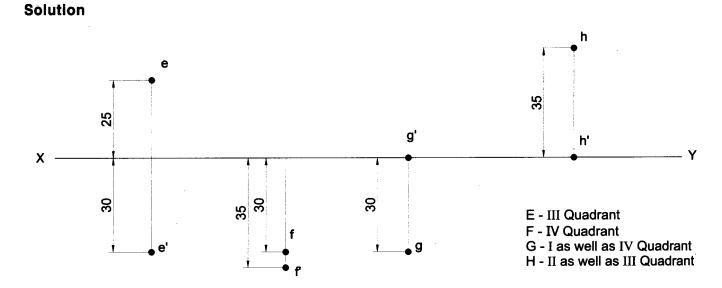
**Problem 3** Draw and state the quadrants in which the following Points are located. Assume any distances. A – Front view below XY line & Top view above XY line.
