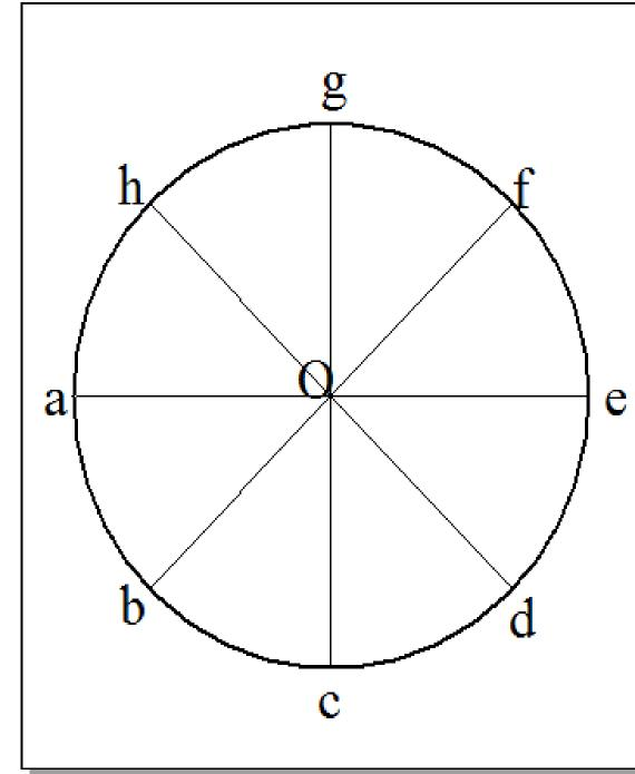
1. Construct circle by circle by center point command. 2. Draw a line oe 3. Select the line oe 4. Click on Circular Pattern command. e 5. Type No. of Count = 8 and Angle = 3606.Click at center point O and then click on Finish button.
