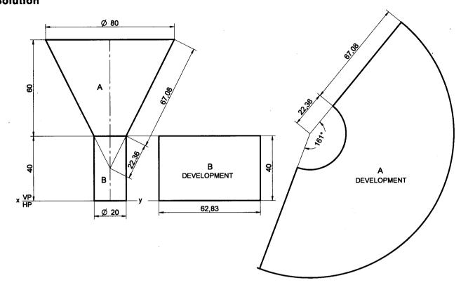
**Problem 48** Draw the development of the lateral surface of the cut cone, whose front view is shown in the following figure. **Solution**
