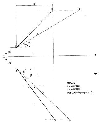
**Problem 32** The top view ab of a straight line AB is 60 mm long and makes an angle of 30<sup>0</sup> with the XY line. The end A is in VP and 30 mm above HP. The end B is 65 mm above HP. Draw the projections of the line AB and determine i) length of the front view ii) its true length and true inclinations with the reference planes. **Solution**
