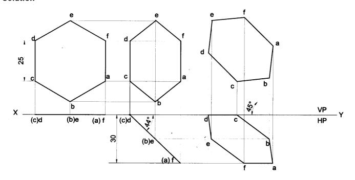
**Problem 45** A hexagonal lamina of sides 25mm rests on one of its corners on HP. The corner opposite to the corner on which it rests is 35mm above HP and the diagonal passing through the corner on which it rests is inclined at 30° to VP. Draw its projections. Find the inclination of the surface with HP. **Solution**
