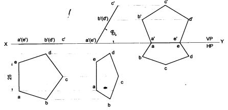
**Problem 25** A pentagonal lamina of sides 25mm is having a side both on HP and VP. The surface of the lamina is inclined at an angle of 60° with HP. Draw the top and front views of the lamina. **Solution**
