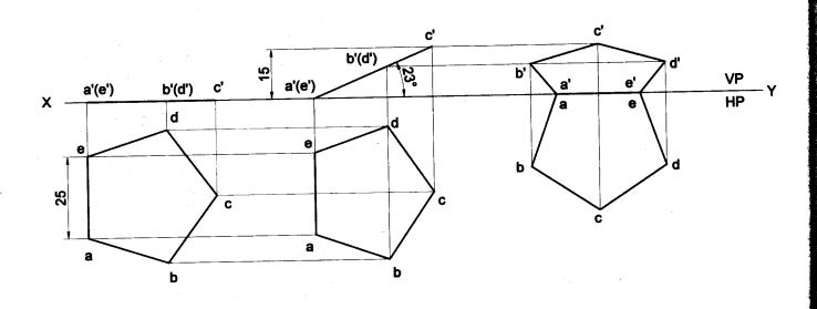
**Problem 26** A regular pentagonal lamina of 25mm side is resting on one of its corners on HP while the side opposite to this corner touches VP. If the lamina makes an angle of 60° with HP and 30° with VP, draw the projections of the lamina.
