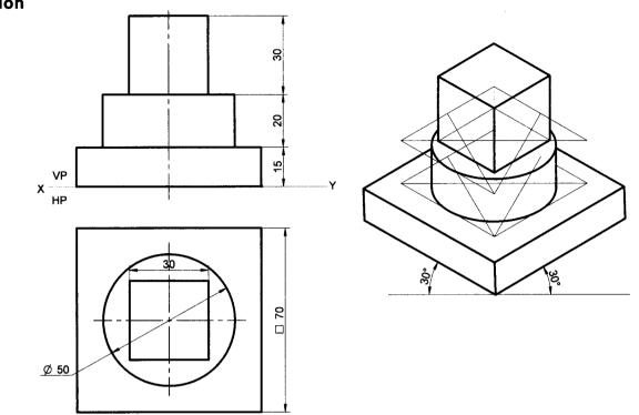
**Problem 32** Following figure shows the front and side views of solid. Draw the Isometric projection of the solid. **Solution**
