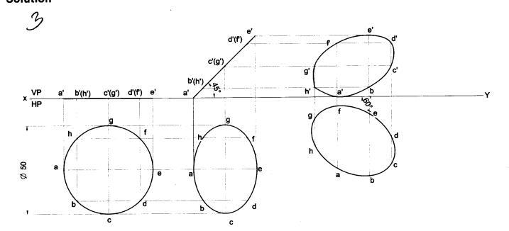
**Problem 47** A circular lamina of 50mm diameter is standing with one of its points on the rim on HP and the lamina inclined at 45° to HP. The diameter at right angles to the diameter which is passing through the point on which the lamina rests is parallel to VP. Draw its projections. **Solution**
