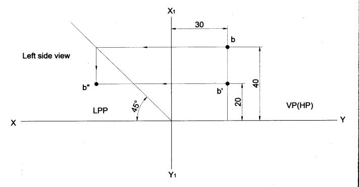
Problem 44 A point is 30 mm behind VP, 30 mm above HP and 25 mm in front / behind / from RPP. Draw its projections and name the side views. Solution
