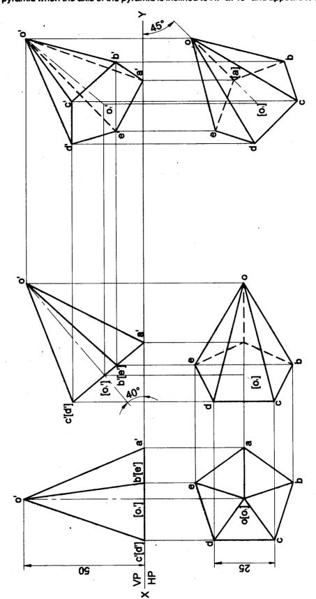
**Problem 23** A pentagonal pyramid 25 mm sides of base and 50 mm axis length rests on HP on one of its corners of the base such that the two base edges containing the corner on which it rests make equal inclinations with HP. Draw the projections of the pyramid when the axis of the pyramid is inclined to HP at 40° and to VP at 30°. **Solution**
