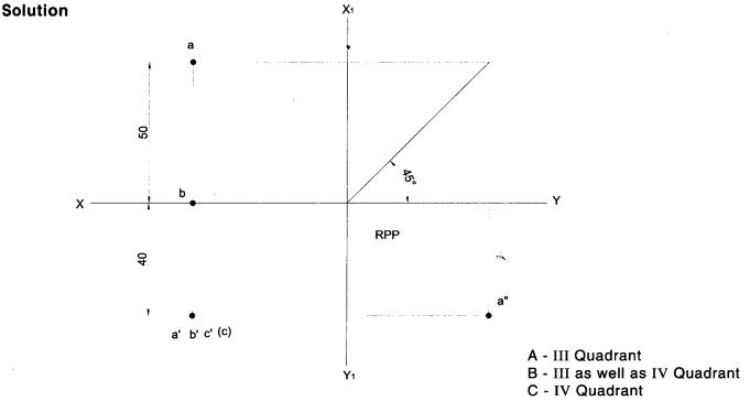
**Problem 31** A point A is on HP and 35 mm in front of VP. Another Point B is on VP and below HP. The line Joining their front views makes an angle of 30 deg to XY line while the line joining their top views makes an angle 45 deg with XY line. Find the distance of the point B from HP. Solution
