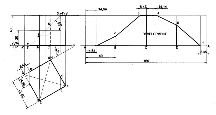
**Problem 6** A square prism of base side 35mm rests with its base on HP and two faces equally inclined to VP. Draw the development of the lateral surfaces of the retained portions of the cut prism shown by dark lines in the Fig. **Solution**
