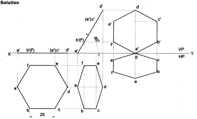
**Problem 38** A hexagonal lamina of sides 30mm is resting on HP with one of its corners in VP and its surface inclined at an angle of 30° with VP. The diagonal passing through that corner which is in VP is inclined at 45° to HP. Draw the projections of the lamina. **Solution**
