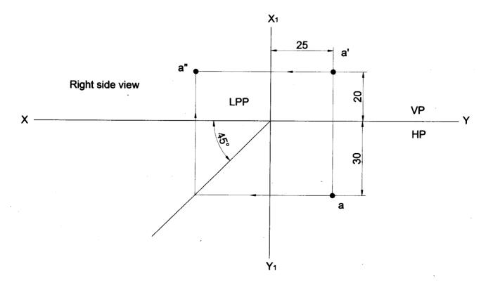
Problem 43 A point is 40 mm behind VP, 20 mm above HP and 30 mm in front / behind / from LPP.Draw its projections and name the side view.
