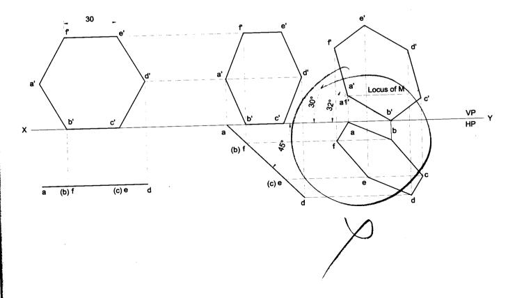
**Problem 33** Draw the top and front views of a hexagonal lamina of 30mm sides having two of its edges parallel to both vertical and horizontal planes and one of its edges is 10mm from each of the planes of projection. The surface of the lamina is inclined at an angle of 60° to the HP. **Solution**
