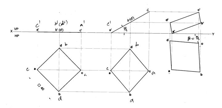
**Problem 11** The top view of a square lamia of side 30mm is a rectangle of sides 30mm x 20mm with the longer side of the rectangle being parallel to both HP and VP. Draw the top and front views of the square lamina. What is the inclination of the surface of the lamina with HP and VP? **Solution**
