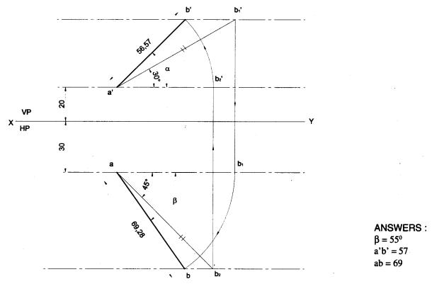
Problem 2 A line AB 80 mm long is inclined to HP at 30° and inclined to VP at 45°. Draw front and top views of line and determine their lengths. Also measure the perpendicular distance of end B from both HP and VP. Solution
