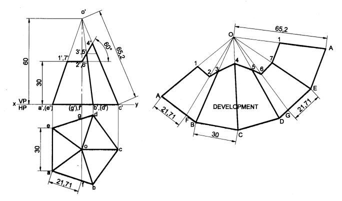
**Problem 26** A pentagonal pyramid of 30mm edges of base and 50mm height rests vertically with one of its base edges parallel to VP and nearer to it. It is cut as shown in following figure. Draw the development of the lateral surfaces of the upper portion of the pyramid. **Solution**
