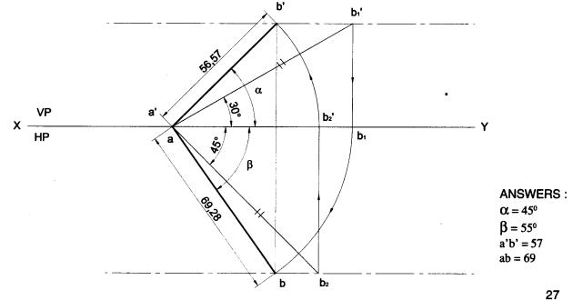
**Problem 3** A line AB has its end A 20 mm above the HP and 30 mm infront of the VP. The other end B is 60 mm above the HP. The distance between end projectors is 70 mm. draw its projections. Determine the true length and apparent inclinations.
