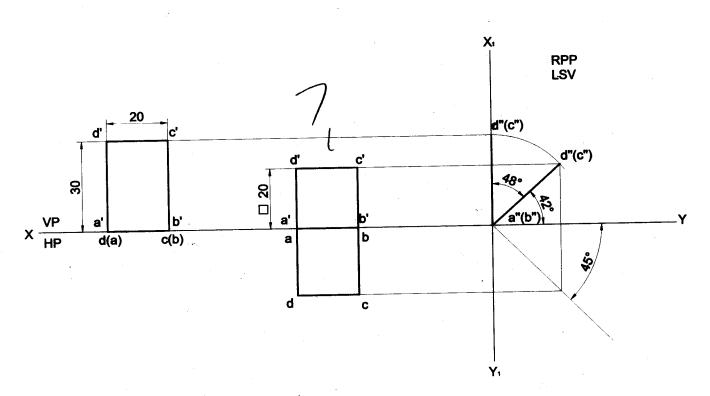
**Problem 17** A mirror 30mm x 40mm is inclined to the wall such that its front view is a square of 30mm side. The longer sides of the mirror appear perpendicular to both HP and VP. Find the inclination of the mirror with the wall. **Solution**
