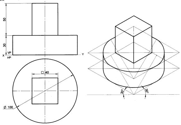
**Problem 21** A square prism base side-40mm, height50mm is placed centrally on a rectangular slab sides-100mmx60mm and thickness-20mm. Draw the isometric projection of the combination **Solution**
