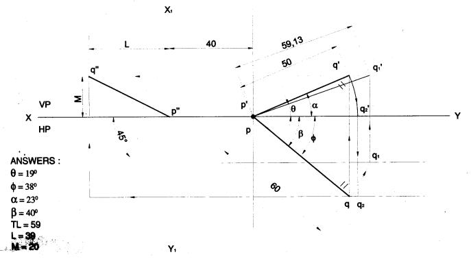
**Problem 26** A line has one end 30 mm in front of VP and 15 mm above HP and the other end is 15 mm in front of VP and is above HP. Length of the line is 60 mm. Top view of the line is 40 mm long. Draw the two views of the line and obtain the inclination of the line with HP and VP. **Solution**
