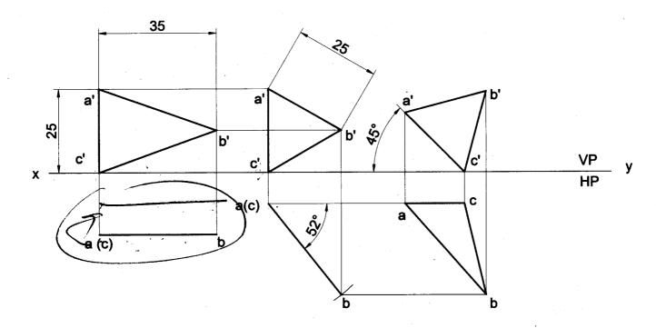
Problem 8 A square lamina of 40mm side rests on one of its sides on HP. The lamina makes 30° to HP and the side on which it rests makes 45° to VP. Draw its projections. Solution
