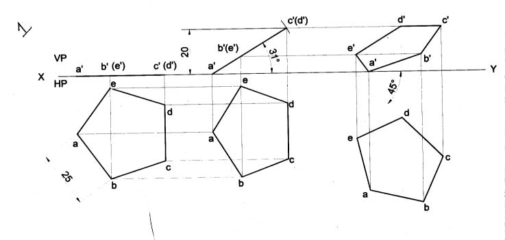
**Problem 22** A pentagonal lamina of sides 25mm is resting on one of its edges on HP with the corner opposite to that edge touching VP. This edge is parallel to VP and the corner, which touches VP, is at a height of 15mm above HP. Draw the projections of the lamina and determine the inclinations of the lamina with HP and VP and the distance at which the parallel edge lies from VP.
