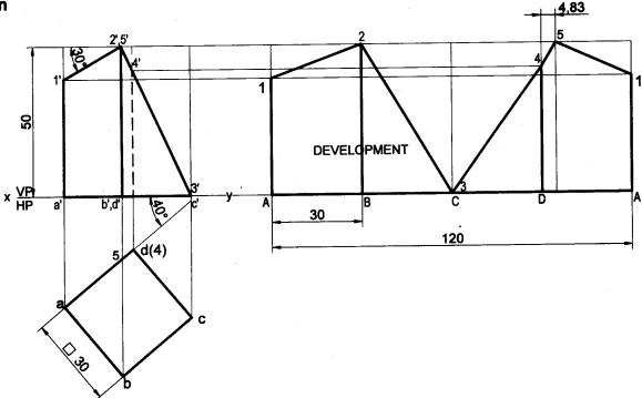
**Problem 5** A cube of side 40mm is resting on HP with its base on HP such that one of its vertical faces is inclined at 30° to the VP. It is cut by a section plane perpendicular to VP, inclined to HP at an angle 45° and passes through the midpoint of the axis. Draw the development of the lower lateral surface of the cube. **Solution**
