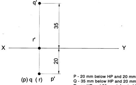
P - 20 mm below HP and 20 mm infront of VP, IV Quadrant Q - 35 mm below HP and 20 mm infront of VP, I Quadrant R - on HP and 20 mm infront of VP, Iaswell as IV Quadrant
