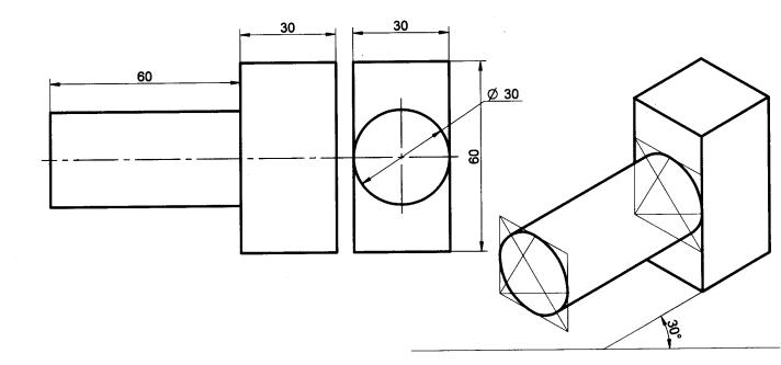
**Problem 29** Following figure shows the front and side views of solid. Draw the Isometric projection of the solid. **Solution**
