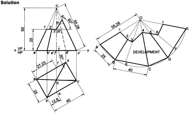
**Problem 23** A frustum of a pentagonal pyramid, smaller base sides 16mm and bigger top face sides 32mm and height 40mm, is resting on the HP on its smaller base, with one of its base sides parallel to the VP. Draw the projections of the frustum and develop the lateral surface it. **Solution**
