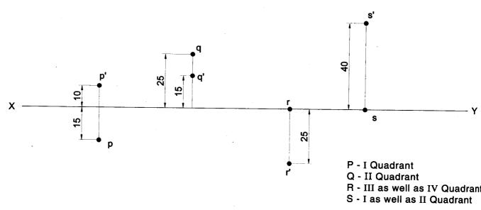
**Problem 36** A point P is 25 mm above HP & 20 mm in front of VP. Another point Q is on HP and 30 mm behind VF. The distance between their projectors measured parallel to the line of intersection of VP and HP is 50mm. Find the distance between the top views of points P and Q. **Solution**
