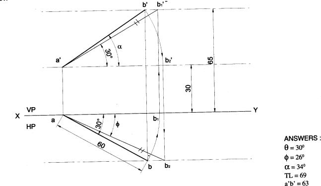
**Problem 33** A line AB 65 mm long, has its end A 25 mm above HP and 30 mm in front of VP. The other end is 45 mm above HP and 50 mm in front of VP. Draw the projections and determine its inclinations. **Solution**
