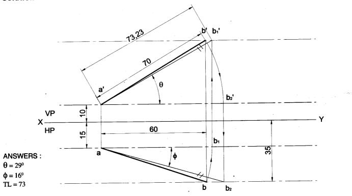
**Problem 13** The distance between the end projectors through the end points of a line AB is 40 mm. The end A is 20 mm above HP and 15 mm in front VP. The end B is 45 mm infront of VP. The line AB appears 50 mm long in the front view. Complete the projections. Find the true length of the line and its inclinations with HP and VP. **Solution**
