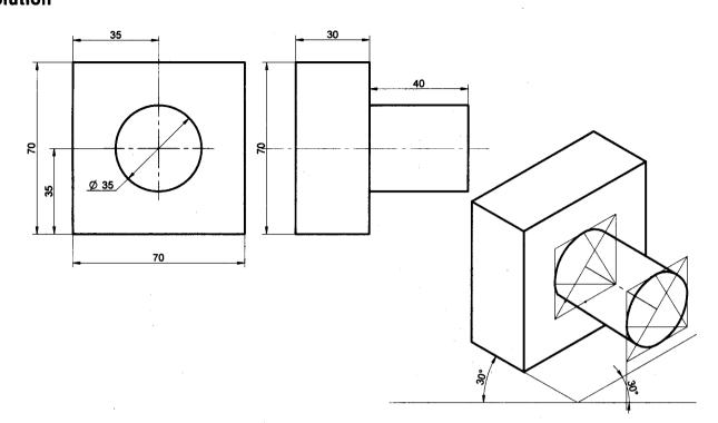
**Problem 30** Following figure shows the front and top views of solid. Draw the Isometric projection of the solid.
