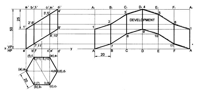
**Problem 16** A hexagonal prism of base side 25mm and height 55mm is resting on HP on its base, such that one of its base edges is parallel to VP. The prism is cut in this position as shown in the following front view. Draw the development of the lateral surface of the prism. **Solution**
