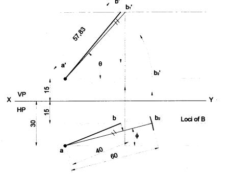
ANSWERS :  $\theta = 48^{\circ}$  $\phi = 14^{\circ}$  **Problem 27** The top view of line PQ 75 mm long measures 50 mm. The end P is 30 mm in front of VP and 15 mm above HP. The end Q is 15 mm in front of VP and above HP. Draw the Projections of the line and find its true inclinations with HP and VP. Find the length of front view and distance between the end Projectors. **Solution**
