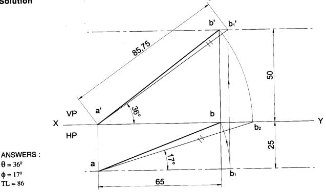
**Problem 45** A line has its end A, 15mm from HP & 10 mm from VP. The end B is 55mm from HP and the line is inclined at 30° to HP. The distance between the end projectors is 50mm. Draw the projections of the line. Determine the true length of the line and its inclination with VP. **Solution**
