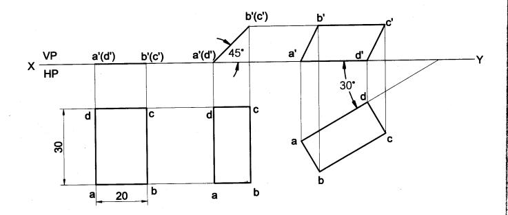
**Problem 13** A rectangular lamina of 35mm x 20mm rests on HP on one of its shorter edges. The lamina is rotated about the edge on which it rests till it appears as a square in the top view. The edge on which the lamina rests being parallel to both HP and VP. Draw its projections and find its inclinations to HP and VP. **Solution**
