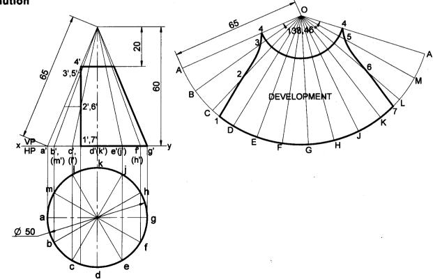
**Problem 49** A funnel is to be made of sheet metal. The funnel tapers from 40 mm to 20 mm diameter to a height of 20 mm and from 20 mm to 15 mm diameter, for the next 20 mm height. The bottom of the funnel is beveled off to a plane inclined at 45° to the axis. Draw the development of the funnel. **Solution**
