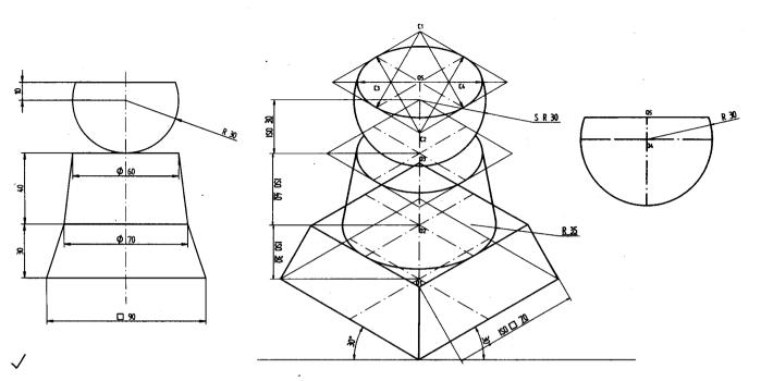
**Problem 6** The frustum of a square pyramid of sides 40mm and height 60mm rest on the centre of the top of a square block of side 60mm and height 20mm. The base edges of the pyramid are parallel to the top edges of the square block. Draw the isometric projection of the combination of the solids. **Solution**
