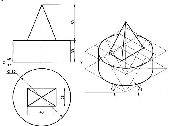
**Problem 19** A rectangular pyramid of base-40mmx25mm and height50mm is placed centrally on a rectangular slab sides-100mmx60mm and thickness-20mm. Draw the isometric projection of the combination **Solution**
