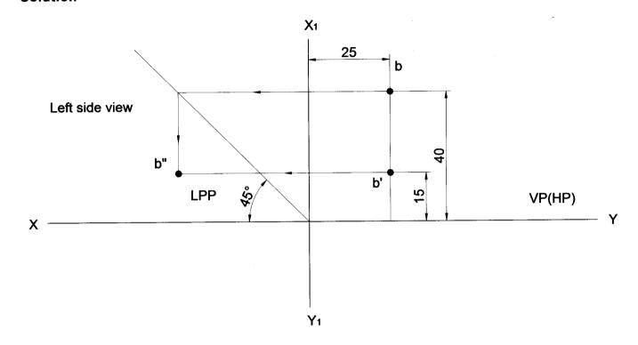
**Problem 20** A point is 30 mm behind VP, 30 mm above HP and 25 mm in front / behind / from LPP. Draw its projections and name the side view. **Solution**
