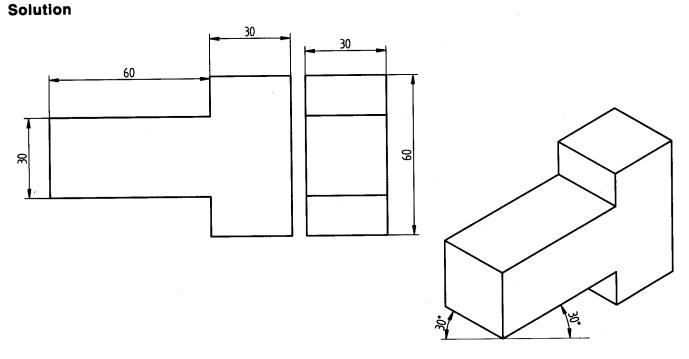
**Problem 28** Following figure shows the front and side views of solid. Draw the Isometric projection of the solid.
