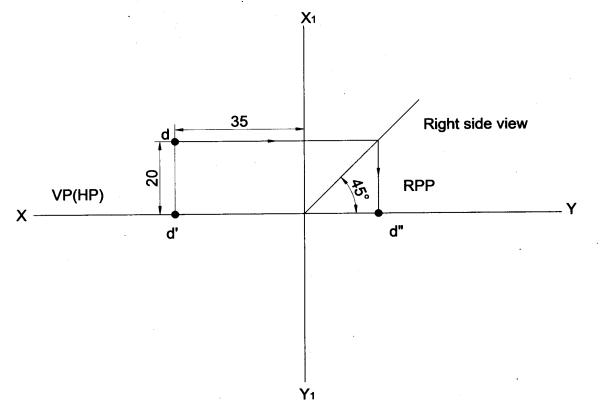
**Problem 47** A point is 35 mm below HP, 15 mm behind VP & 25 mm behind / in front / from RPP. Draw its projections and name the side view. **Solution**
