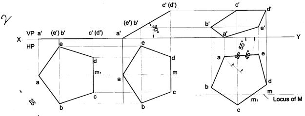
**Problem 24** A pentagonal lamina of sides 25mm is having a side both on HP and VP. The corner opposite to the side on which it rests is 15mm above HP. Draw the top and front views of the lamina. **Solution**
