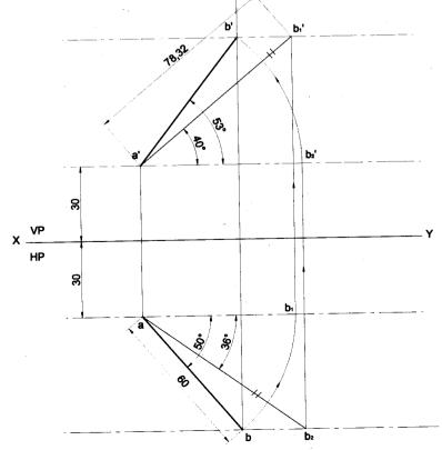
ANSWERS :  $\phi = 36^{\circ}$ TL = 78 Problem 35 The top view of the line AB 80 mm long, measures 65 mm. The mid point of the line is 60 mm in front of VP and 70 mm above HP. The point A is in the VP. Draw its projections and find its inclinations. Solution
