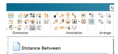
Creates a linear distance dimension between elements or keypoints on the model.
