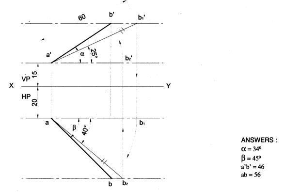
**Problem 10** A line AB measuring 70 mm has its end A 15 infront of VP and 20 mm above HP and the other end B is 60 infront of VP and 50 mm above HP. Draw the projections of the line and find the inclinations of the line with both the reference planes of projection. **Solution**
