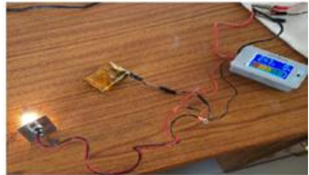
Fig.6 Discharging of graphene battery.
