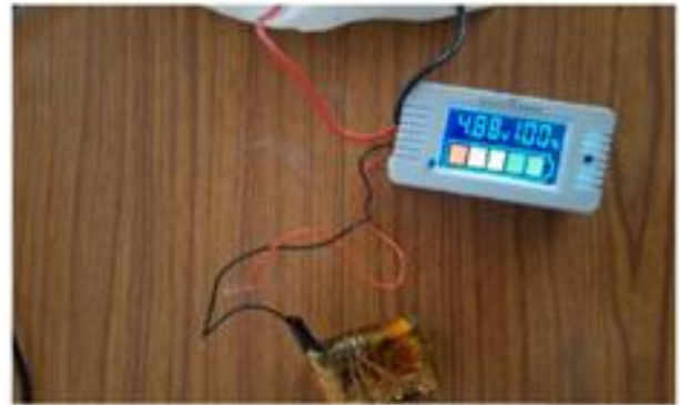
Fig.7 Fully charged graphene battery with voltage of 4.88 V
