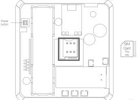
After inserting the SIM card and powering on your GT001-N, put the top lid back to its original position and push it down to close.
