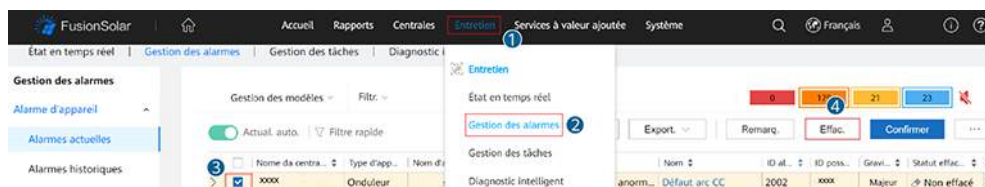
Figure 7-13 Effacement des alarmes
