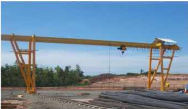
GANTRY CRANE CAP 5 TON X 20 Meter SPAN x 60 Meter Long Travel ( 1 UNIT )
