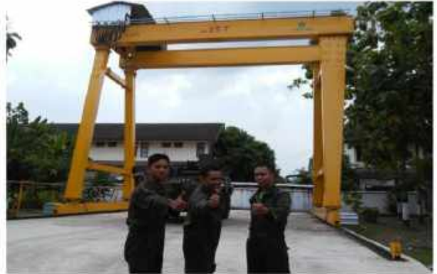
PAWELL DOUBLE GIRDER Gantry CRANE CAP 25TON X 12Meter SPAN x 35Meter Long Travel ( 1UNIT )
