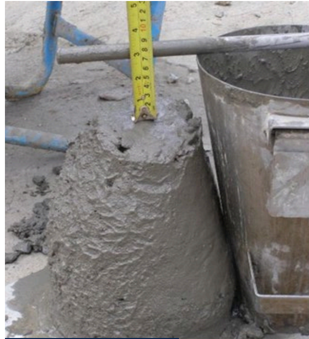
True Slump Zero Slump Collapsed Slump Shear Slump potentially non-plastic potentially non-cohesive no displaced center
