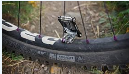
Figure 10. Using a spoke wrench
