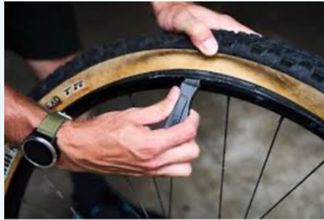
Figure 5. Using tire levers
