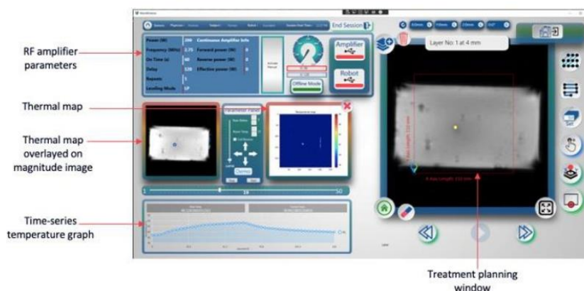
Screenshot of the in-house software platform providing MR thermometry monitoring.
