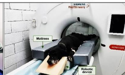
The SOUNDPET device integrated with the SOMATOM CT scanner (Siemens) at V3ts Veterinary Clinic.
