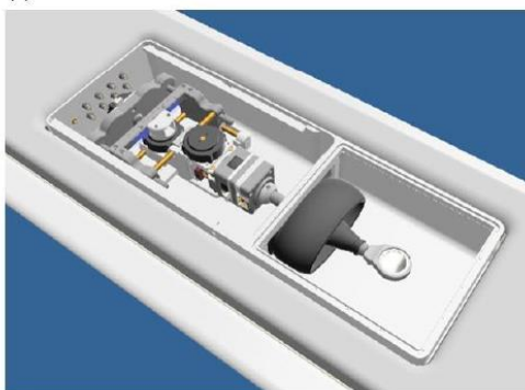
a) Robotic system placed in the MRI with visible mechanism, b) Cross section of the MRI scanner with robot.
