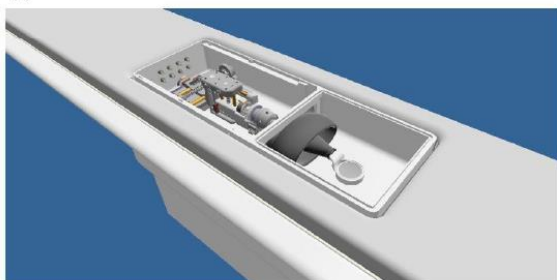
a) CAD drawing of the robotic device as placed in the MRI table, b) Cross section of the device with the dog placed in prone position.
