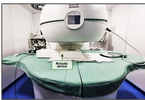
SOUNDPET device placed within the Vet-MR Grande veterinary MRI system (Esaote) at V3ts Veterinary Clinic (Larnaca, Cyprus).
