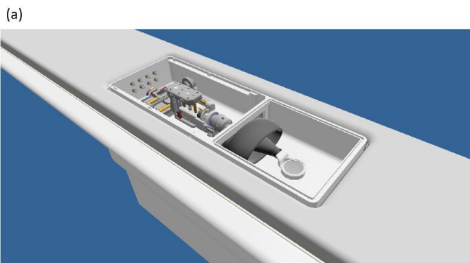
a) CAD drawing of the robotic device as placed in the MRI table, b) Cross section of the device with the dog placed in prone position.
