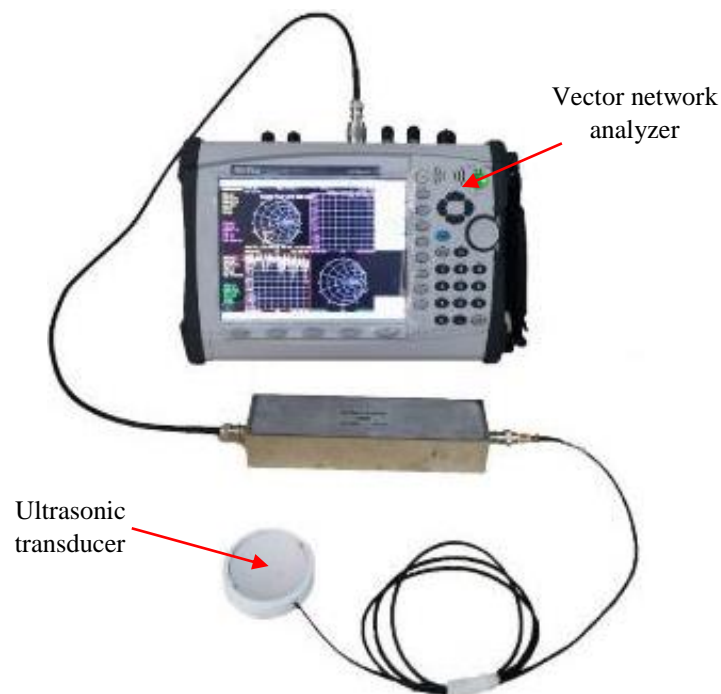
Figure 19: Transducer's impedance measurement without the matching network.
