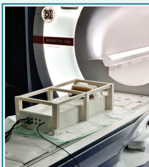
Experimental setup for phantom sonication in the 3T MRI scanner.
