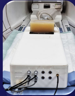
Experimental setup for phantom sonication.
