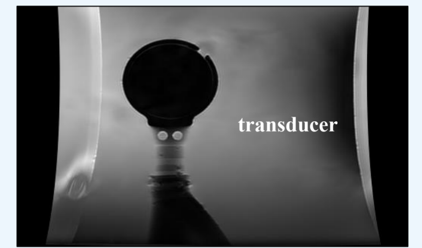
T2-W TSE image (TR = 2500 ms, TE = 52 ms, FA = 180°, ETL = 12, FOV = 260 x 260 x 10 mm 3 , matrix size = 128 x 128, and NEX = 2).
