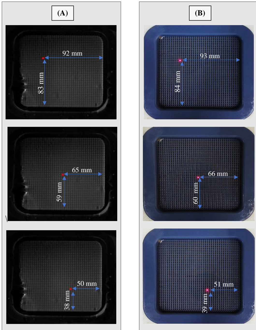
Figure 12: Column (A): Random grid cells selected on the software (3 different locations: No. 9, No. 17, No. 6 of Table 1). Column (B): The laser location after motion execution (3 different locations).
