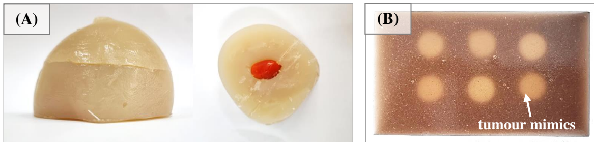
Figure 14: Photos of the (A) Breast-shaped agar-based phantom (6 % w/v agar) featuring a cherry tomato: Isometric view (left) and Cross-section view (right), and (B) agar-based phantom with six biopsy targets.
