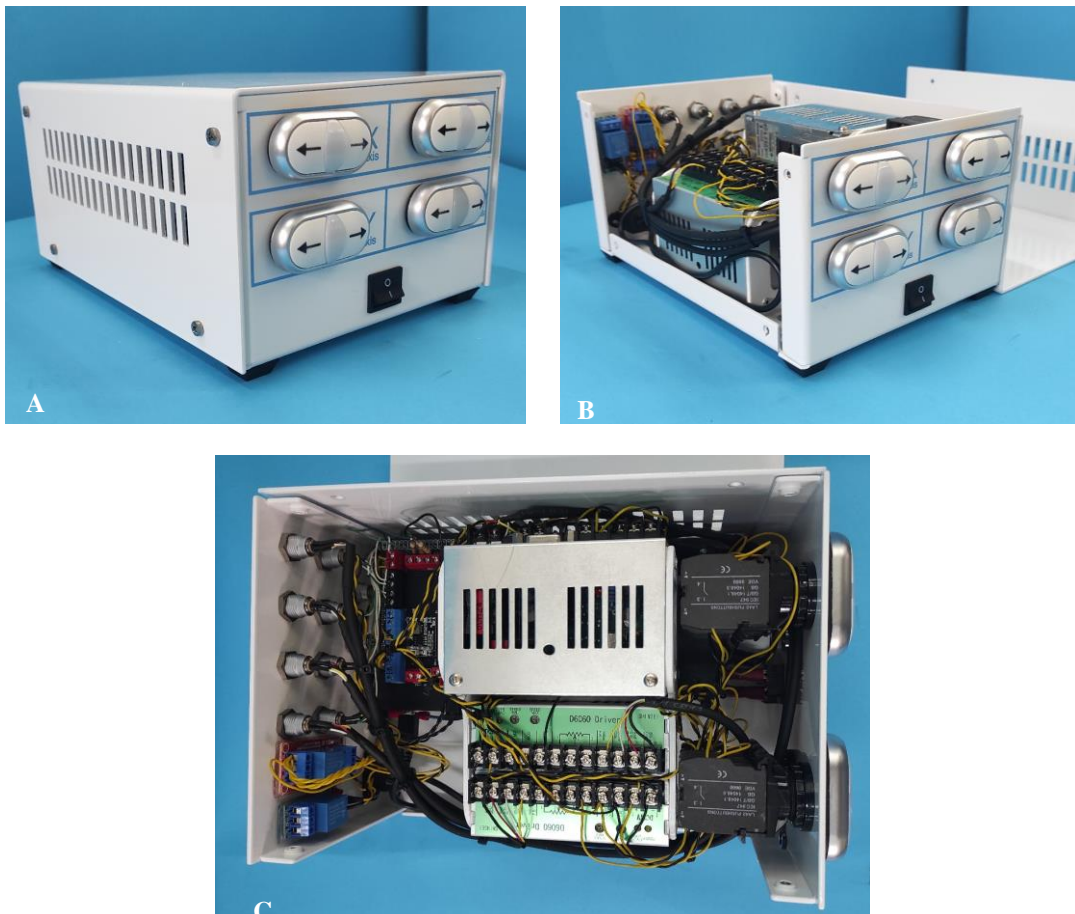
Figure 6: (A) The electronic driving system enclosed in the constructed housing, (B) The electronic driving system without housing. (C) Top view of the electronic driving system without the housing.
