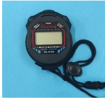
Figure 21: Stopwatch that was used to count the time the robotic system needed to complete the several desired motions.
