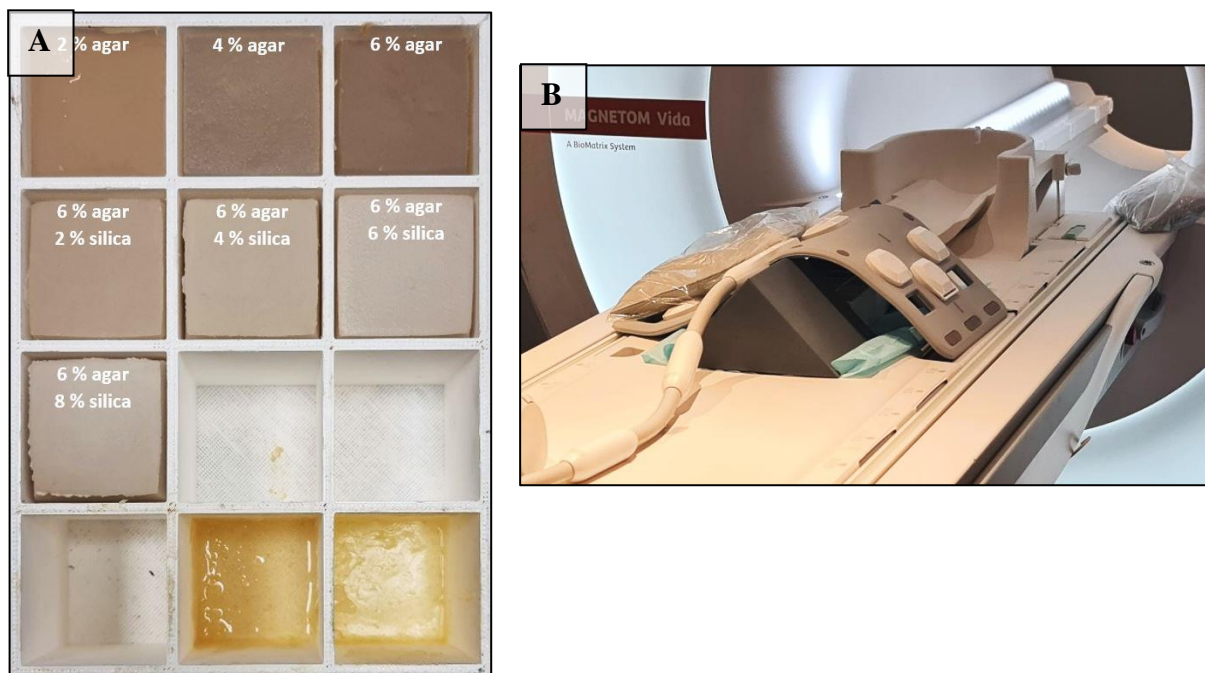
Figure 1: (A) Photo of the phantoms in the container and the corresponding recipe used for each one. (B) The experimental setup for T1 and T2 measurements.
