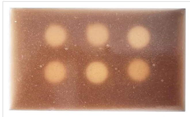
Figure 5: Agar-based phantom with six similar biopsy targets.
