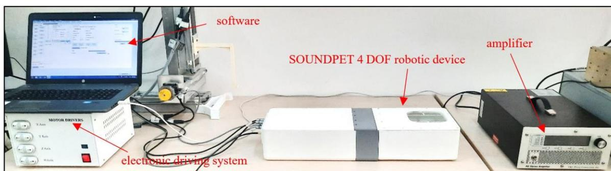
**Figure 3:** Experimental set-up for rabbit thigh ablation.
