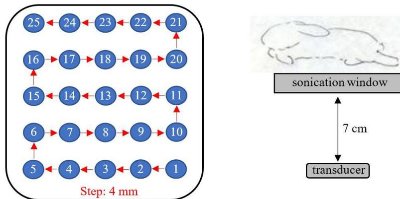
**Figure 2:** Grid movement for ablations on the right thigh and the distance transducer/rabbit thigh.
