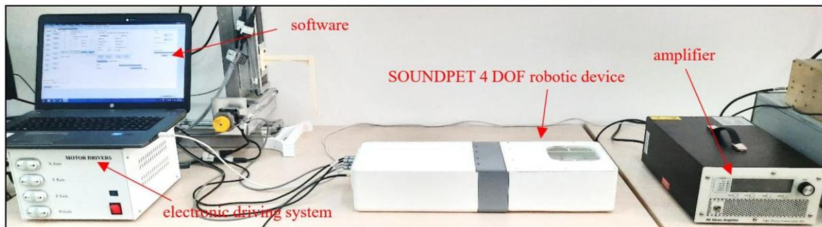
**Figure 2:** Experimental set-up using the 1<sup>st</sup> version of the 4-DOF robotic device.
