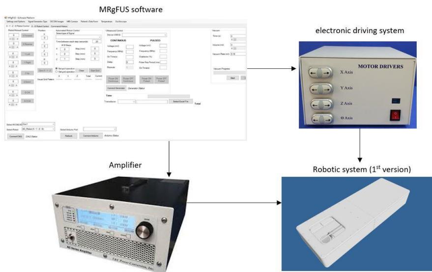
**Figure 1:** Schematic diagram of the experimental set-up using the 1<sup>st</sup> version of the 4-DOF robotic device.
