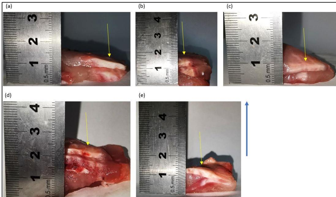
**Figure 12:** Sample images after cross-section of overlapping lesions inflicted by ablation with the SOUNDPET system (version 1) on a plane parallel to the ultrasound beam ( $f = 1.1$  MHz,  $D = 50$  mm,  $R = 70$  mm) for a grid pattern of (a, b, c)  $3 \times 3$ , (d)  $4 \times 4$ , and (e)  $5 \times 5$ . The yellow arrows indicate the ablated area and the blue arrow indicates the ultrasonic beam direction.
