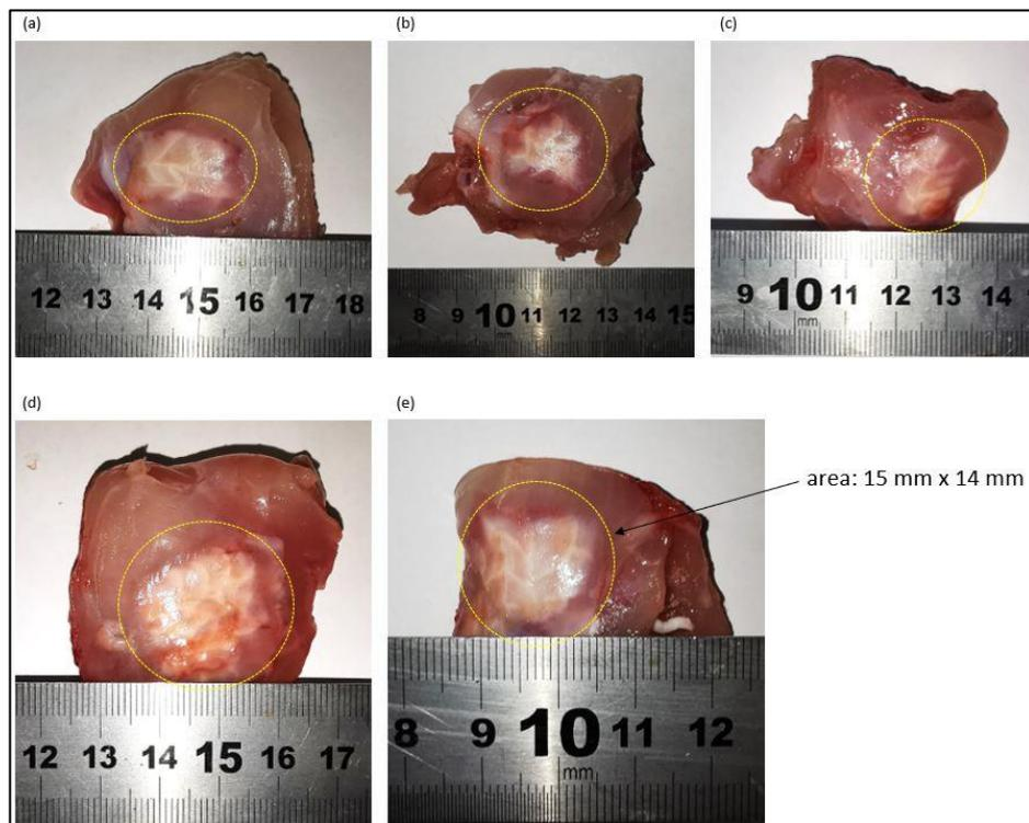
**Figure 11:** Sample images of overlapping lesions inflicted by ablation with the SOUNDPET system (version 1) on a plane perpendicular to the ultrasound beam ( $f = 1.1$  MHz,  $D = 50$  mm,  $R = 70$  mm) for a grid pattern of (a, b, c)  $3 \times 3$ , (d)  $4 \times 4$ , and (e)  $5 \times 5$ . The yellow circles indicate the ablated area.
