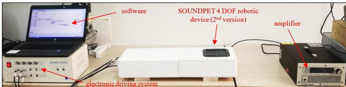
**Figure 3:** Experimental set-up for rabbit thigh ablation.
