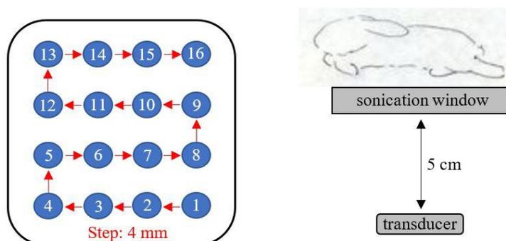
**Figure 2:** Grid movement for ablations on the right thigh and the distance transducer/rabbit thigh.
