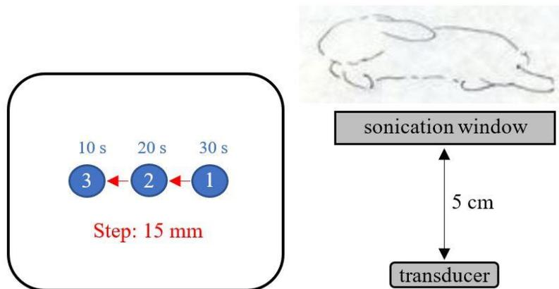
**Figure 2:** Grid movement for ablations on the right thigh and the distance transducer/rabbit thigh.
