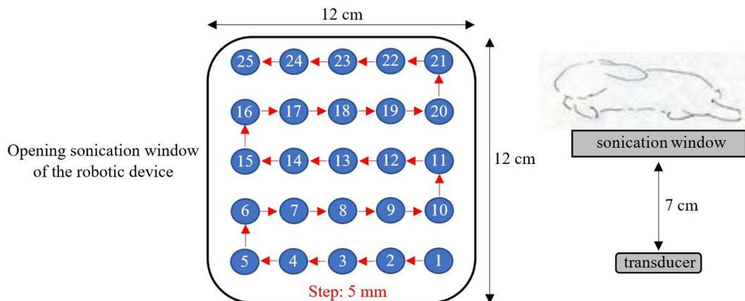
**Figure 1:** Grid movement for ablations on the left thigh and the distance transducer/rabbit thigh.
