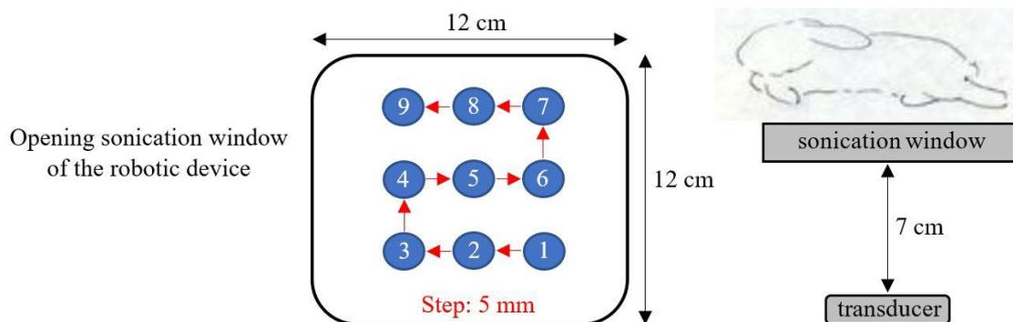
**Figure 1:** Grid movement for ablations on the left thigh and the distance transducer/rabbit thigh.
