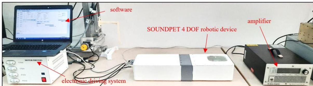
**Figure 3:** Experimental set-up for rabbit thigh ablation.
