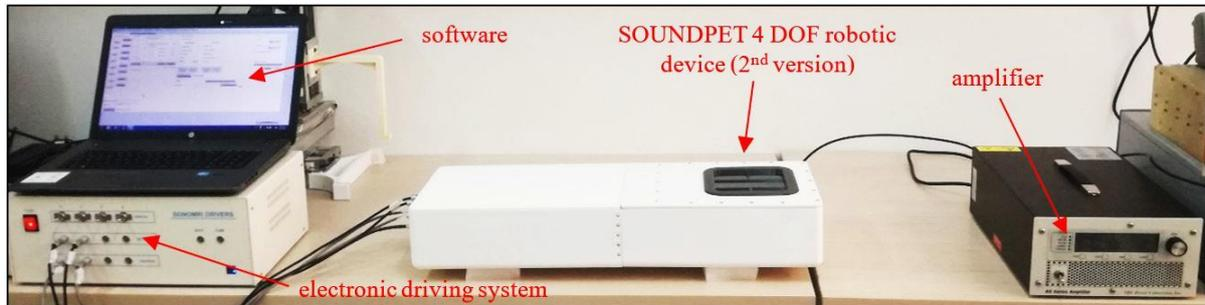
**Figure 2:** Experimental set-up for rabbit thigh ablation.
