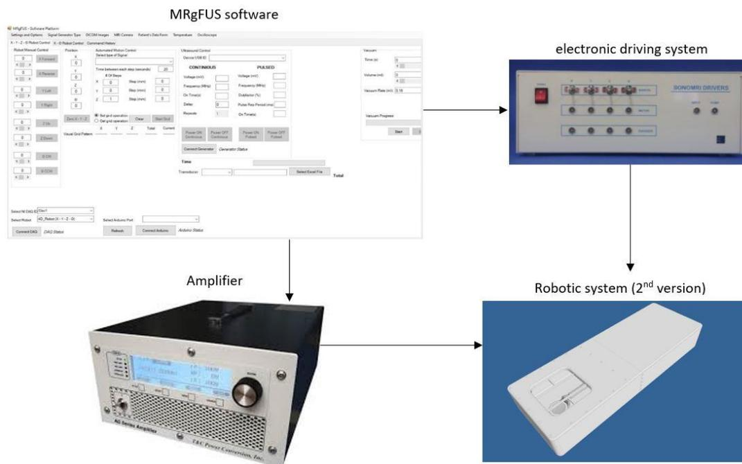
**Figure 133:** Schematic diagram of the experimental set-up using the 4-DOF robotic device (2<sup>nd</sup> version).
