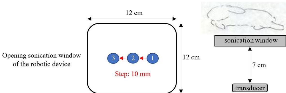
**Figure 1:** Grid movement for ablations on the left thigh and the distance transducer/rabbit thigh.
