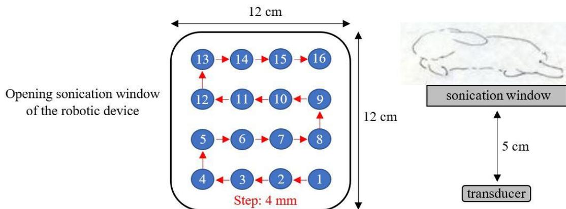
**Figure 1:** Grid movement for ablations on the left thigh and the distance transducer/rabbit thigh.
