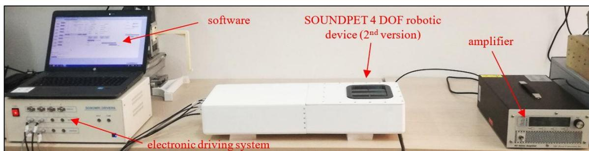
**Figure 14:** Experimental set-up using the 4-DOF robotic device (2<sup>nd</sup> version).
