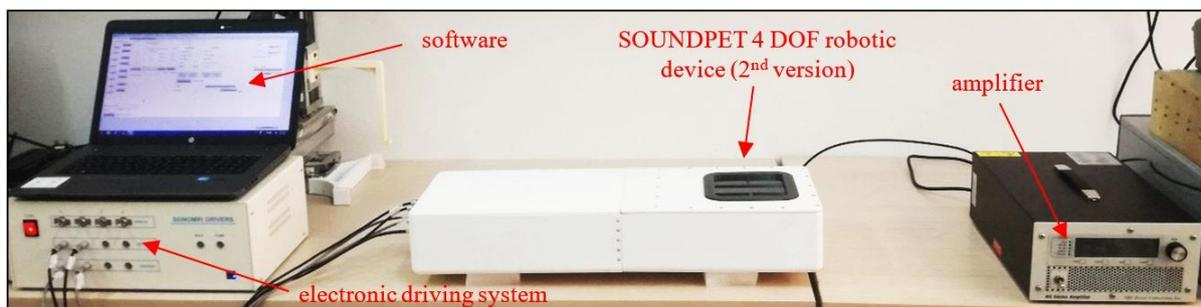
**Figure 1:** Experimental set-up for rabbit thigh ablation.
