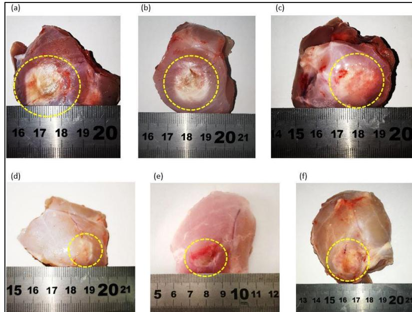
**Figure 19:** Photos of overlapping lesions inflicted by ablation with the SOUNDPET system (version 2) on a plane perpendicular to the ultrasound beam ( $f = 2.6$  MHz,  $D = 38$  mm,  $R = 61$  mm) for a grid pattern of (a, b, d)  $3 \times 3$ , (c, e)  $4 \times 4$ , and (f)  $5 \times 5$ . The yellow circles indicate the ablated area.
