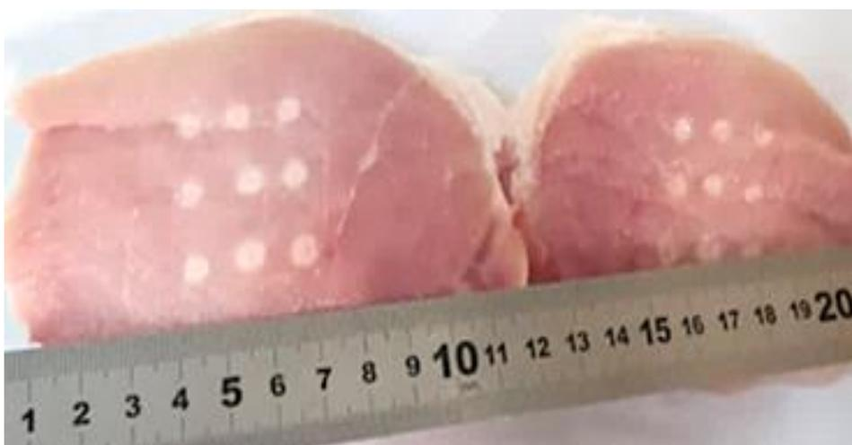
Figure 97: Lesions formed on excised tissue on a plane perpendicular to the beam after exposure at acoustical power of 45 W for a sonication time of 20 s with movement of the 2.75 MHz transducer ( $D=50$  mm,  $ROC=65$  mm) using the robotic device (version 3) in a  $3\times 3$  grid with a 15 mm step at a 25 mm focal depth. Slice of the tissue at 10 mm and its mirror (from left to right).
