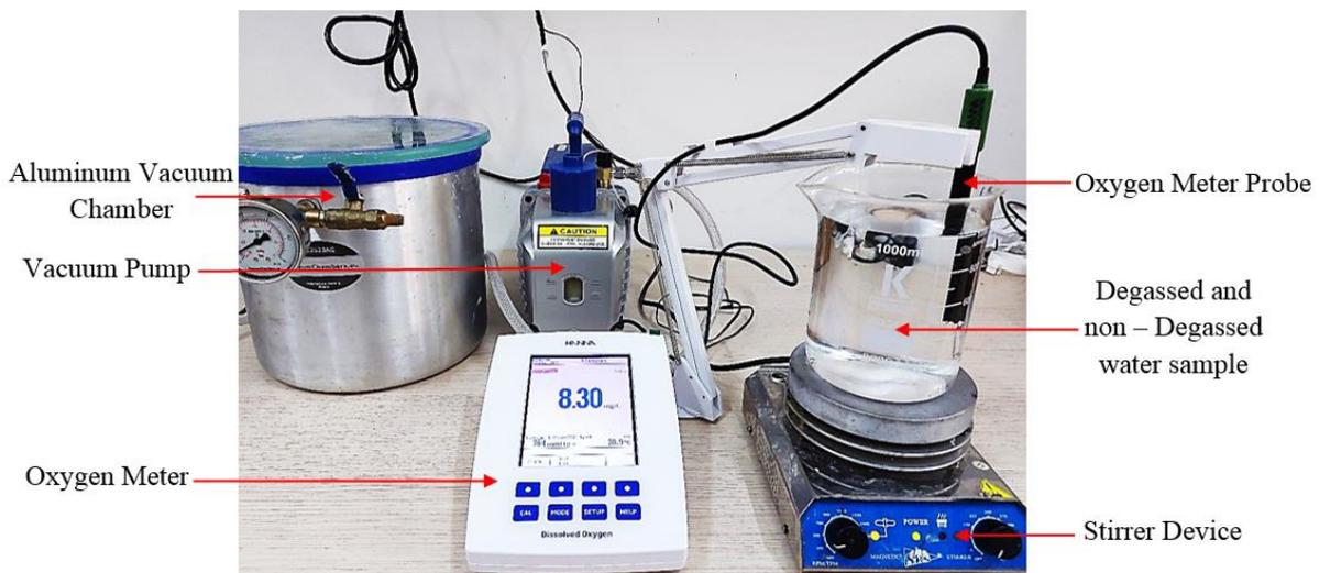
Figure 1: Experimental set-up for measuring the oxygen content of water.
