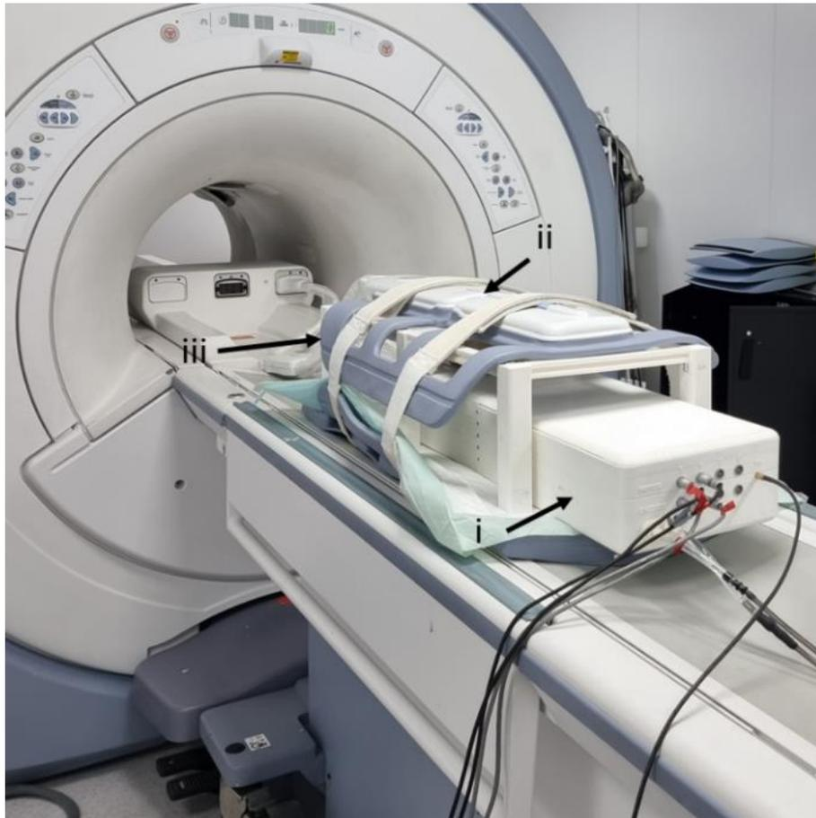
Figure 152: Experimental set-up inside the 1.5 T MRI scanner with the SOUNDPET robot (version 2) (i) positioned on the MRI table with a tumor-like (6 % w/v agar, 4 % w/v silica, 30 % v/v milk) agar-based (4 % w/v agar) phantom (ii) placed on the acoustic window and a body coil (iii) placed on top for MR image acquisition.
