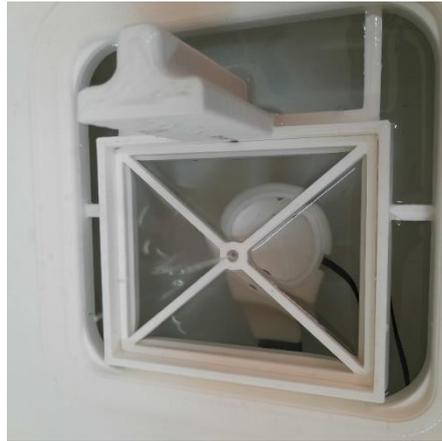
Figure 10: Adjustment of the center of the transducer at the center of the phantom.
