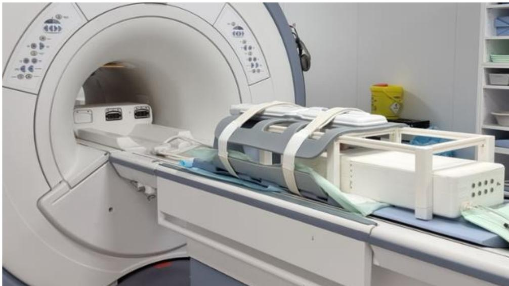
*Figure 163: Experimental set-up inside the 1.5 T MRI scanner with the SOUNDPET robot (version 2) positioned on the MRI table with a piece of excised pork tissue placed on the acoustic window and a body coil accommodated on top for MR image acquisition.*
