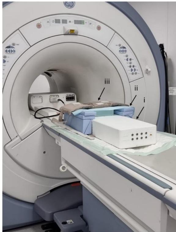
*Figure 119: Experimental set-up inside the 1.5 T MRI scanner with the SOUNDPET robot (version 1) (i) positioned on the MRI table and a piece of excised pork tissue placed on the acoustic window of the robot. Rectangular cushions were placed next to the robot (ii) for supporting the GPFLEX surface coil (iii) that was placed on top for MR image acquisition.*
