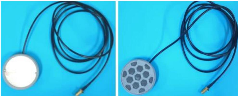
Figure 4: SOUNDPET transducer, frequency = 1.1 MHz, diameter = 60 mm, radius of curvature = 70 mm (MEDSONIC LTD).
