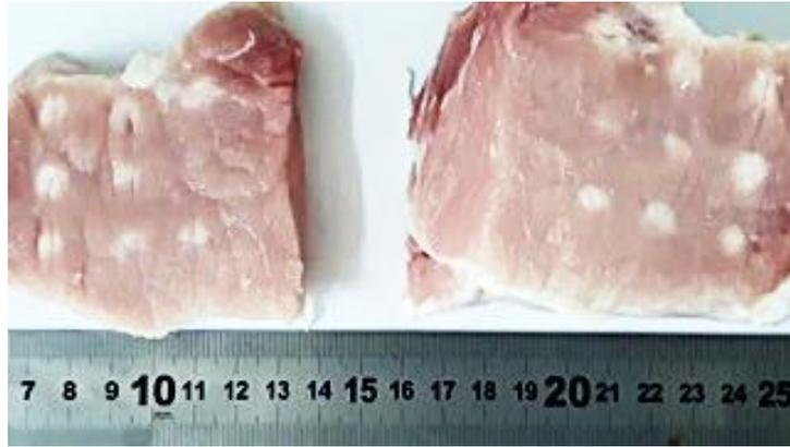
Figure 65: Lesions formed on a plane perpendicular to the beam after exposure at acoustical power of 94 W for a sonication time of 20 s with movement of the 1.1 MHz transducer ( $D=60$  mm,  $ROC=70$  mm) using the robotic device (version 1) in a  $3 \times 3$  grid with a 15 mm step at 10 mm focal depth. Slice of the tissue at 10 mm and its mirror (from left to right).
