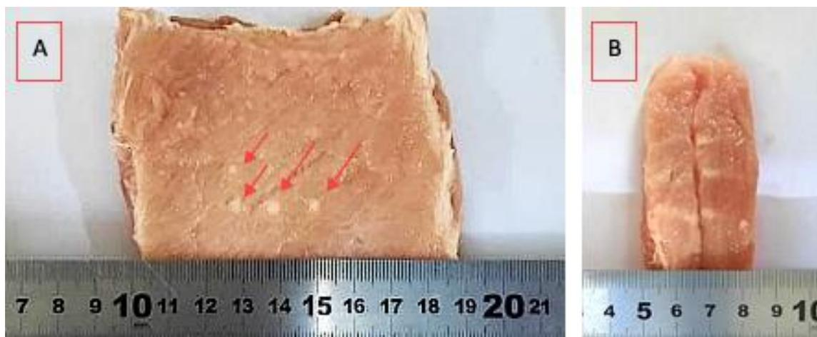
*Figure 64: Lesions formed on excised tissue after exposure at acoustical power of 55 W for a sonication time of 15 s with movement of the 1.1 MHz transducer (D=60 mm, ROC=70 mm) using the robotic device (version 1) in a 3×3 grid with a 10 mm step, with the focal point located at the tissue interface. A) Slice of the tissue at 10 mm showing lesions formed on plane perpendicular to the beam, and B) Lesions formed on a plane parallel to the beam.*
