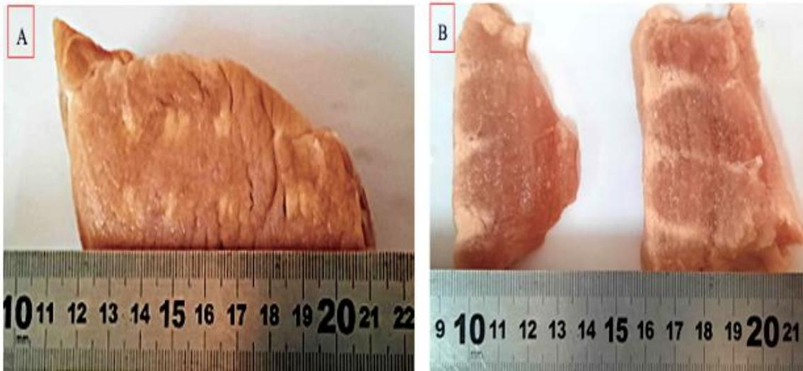
Figure 53: Lesions formed on excised tissue after exposure at acoustical power of 78 W for a sonication time of 20 s, with manual movement of the 1.1 MHz transducer ( $D=60$  mm,  $ROC=70$  mm) in a  $2\times 4$  grid with a 15 mm step, with the focal point located at the tissue interface. A) Lesions formed on plane perpendicular to the beam, and B) Lesions formed on plane parallel to the beam.
