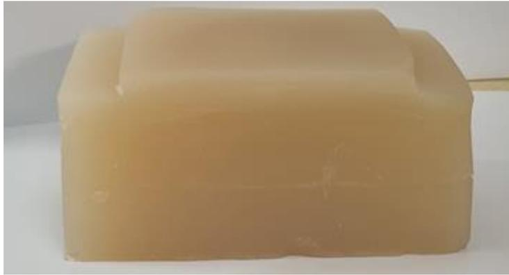
*Figure 156: Agar-based phantom (4 % w/v agar) featuring a tumor-like material (6 % w/v agar, 4 % w/v silica, 30 % v/v milk) in the centre developed with specific shape to allow its support on the acoustic opening of the robotic system.*
