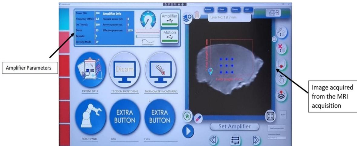
Figure 164: Screenshot of the software used in the experiment allowing treatment planning on MR images and execution of robotic motion based on the planned sonication area.
