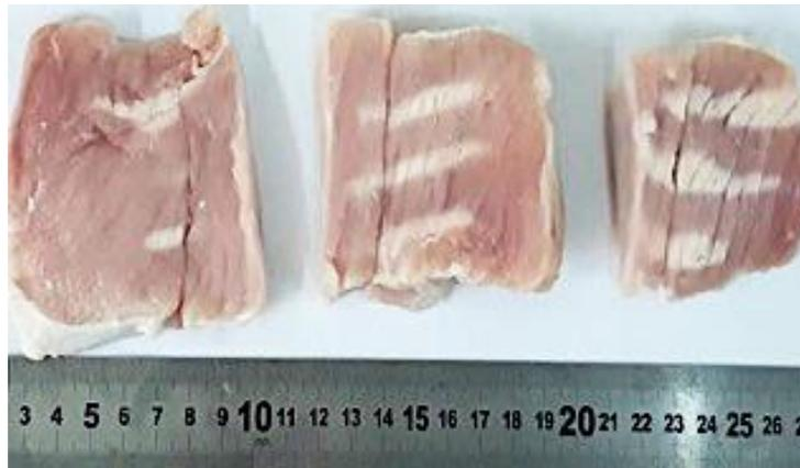
Figure 66: Lesions formed on a plane parallel to the beam after exposure at acoustical power of 94 W for a sonication time of 20 s with movement of the 1.1 MHz transducer ( $D=60$  mm,  $ROC=70$  mm) using the robotic device (version 1) in a  $3 \times 3$  grid with a 15 mm step at 10 mm focal depth.
