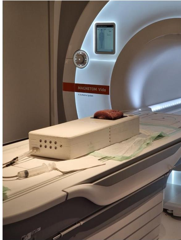
Figure 185: Experimental set-up with the SOUNDPET robot (version 2) positioned on the table of the 3 T MRI scanner with a piece of excised pork tissue placed on the acoustic window for assessing lesion detection using T2-W imaging.
