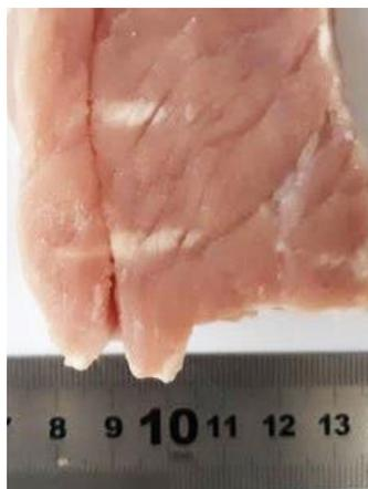
Figure 68: Lesions formed on a plane parallel to the beam after exposure at acoustical power of 109 W for a sonication time of 10 s with movement of the 1.1 MHz transducer ( $D=60$  mm,  $ROC=70$  mm) using the robotic device (version 1) in a 3×3 grid with a 15 mm step at 10 mm focal depth.
