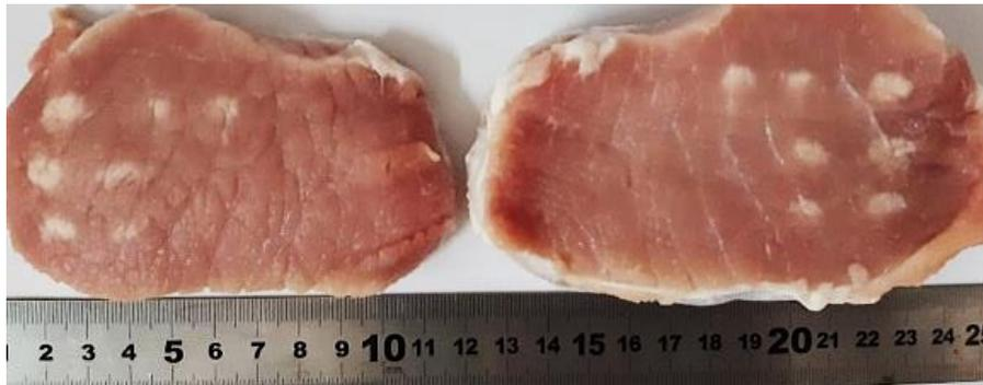
Figure 69: Lesions formed on a plane perpendicular to the beam after exposure at acoustical power of 109 W for a sonication time of 15 s with movement of the 1.1 MHz transducer ( $D=60$  mm,  $ROC=70$  mm) using the robotic device (version 1) in a 3×3 grid with a 15 mm step at 10 mm focal depth. Slice of the tissue at 10 mm and its mirror (from left to right).
