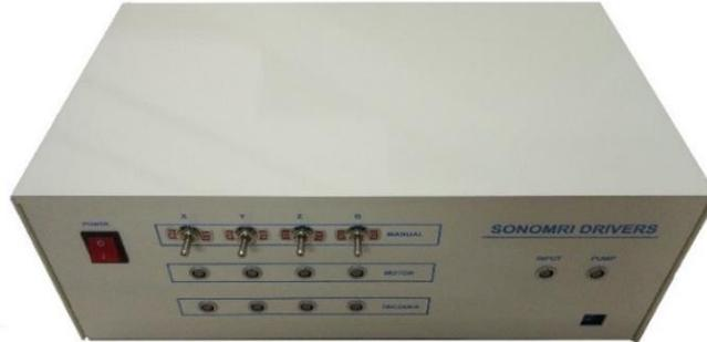
Figure 120: Electronic system for controlling the large USR60-S3N (Shinsei Corporation) motors.
