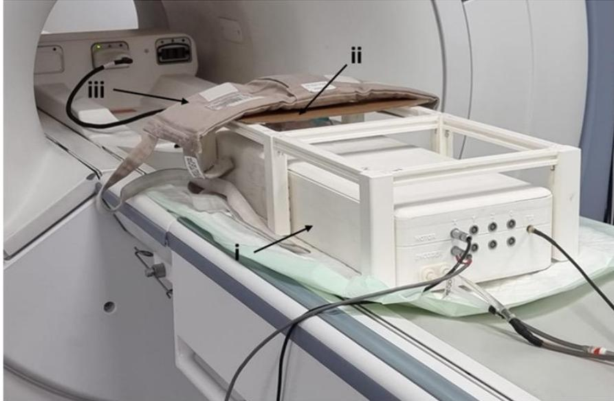
Figure 137: Experimental set-up inside the 1.5 T MRI scanner with the SOUNDPET robot (version 2) (i) positioned on the MRI table and a piece of excised pork tissue (ii) placed on the acoustic window with a plastic positioner accommodated on top for supporting the GPFLEX coil (iii) used for MR image acquisition.
