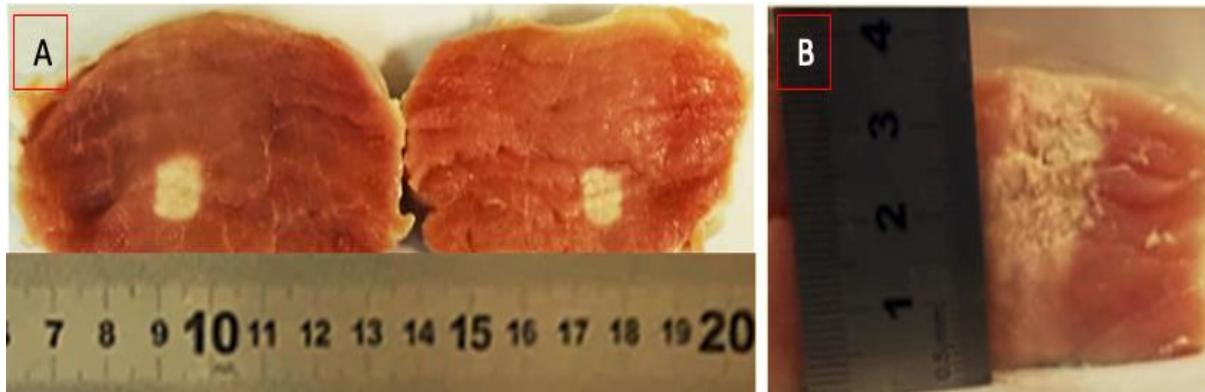
Figure 99: Overlapping lesions formed on excised tissue after exposure at acoustical power of 45 W for a sonication time of 10 s with movement of the 2.75MHz transducer ( $D=50$  mm,  $ROC=65$  mm) in a  $3\times 3$  grid with a 5 mm step at a 25 mm focal depth. A) Lesions formed on plane perpendicular to the beam. Slice of the tissue at 15 mm and its mirror (from left to right), and B) Lesions formed on plane parallel to the beam.
