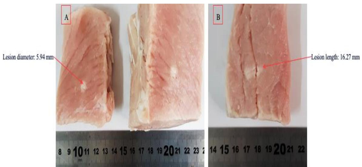
Figure 42: Lesion formed on excised pork tissue after exposure with the 1.1 MHz transducer ( $D=60$  mm,  $ROC=70$  mm) at acoustical power of 74 W for a sonication time of 30 s at 10 mm focal depth. A)
