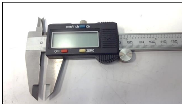
Figure 4: Digital caliper that was used to evaluate the X and Y linear motions of the robotic system.
