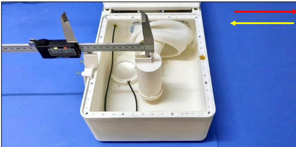
Figure 15: Evaluation of the motion accuracy of the robotic device in the Y-axis. The red arrow indicates the left direction and the yellow arrow indicates the right direction.
