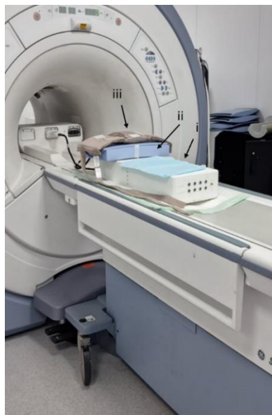
Figure 17. SOUNDPET Robot v2 (i) positioned on the MRI table. A piece of raw meat was placed at the acoustic opening above the US transducer. A rectangular positioner (ii) was used to increase the distance between the transducer and the coil (iii).
