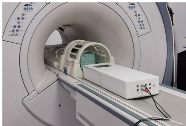
Figure 22. SOUNDPET Robotic System v2 positioned on MRI table. The ACR phantom was placed inside the split head coil close to the robot.
