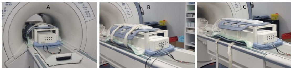
Figure 48. SOUNDPET Robot v3 positioned on the MRI table. An agar-based phantom was placed at the acoustic opening above the transducer. An orthogonal plastic positioner was used to properly position the body coil at sufficient distance above the phantom. (A) Cables disconnected, (B) Cables connected, and (C) Transducer Cable connected.
