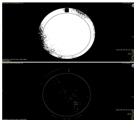
Figure 27. Image of slice 7 showing the large (200 cm 2 ) and the small (1 cm 2 ) ROIs. (Top) Example of measuring the mean signal of low intensity. (Bottom) Example of measuring the mean signal of high intensity.
