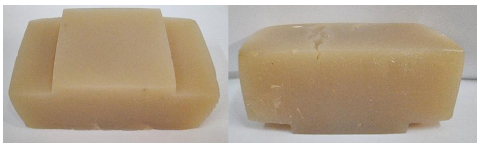
Figure 49. The agar-based phantom (6 % w/v agar) used in the experiment. Its shape was such as its top part was supported on the plastic holder and only its bottom part was submerged into water.
