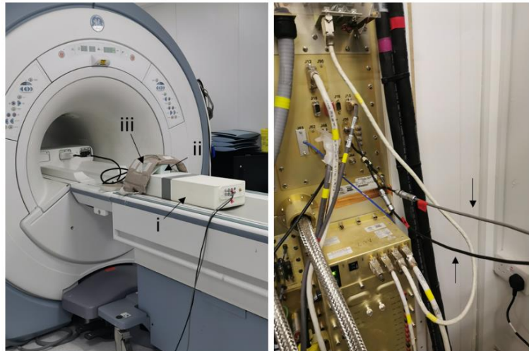
Figure 4. (Left) SOUNDPET Robot v1 (i) positioned on the MRI table. A homogeneous MR phantom (ii) was positioned on the device and covered by the GPFLEX surface coil (iii). (Right) Cables connected on the MRI panel (arrows); cable in black was connected to the motor and cable in grey was connected to the encoder.
