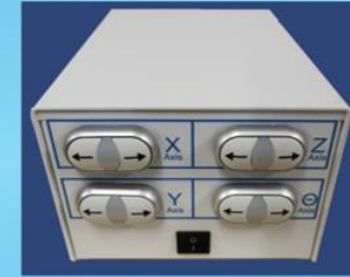
Figure 3: Electronic system that controls the robotic device.
