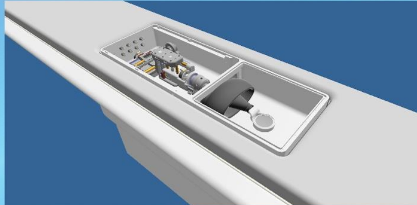
Figure 1: Schematic of the robotic system embedded in the MRI Bed.
