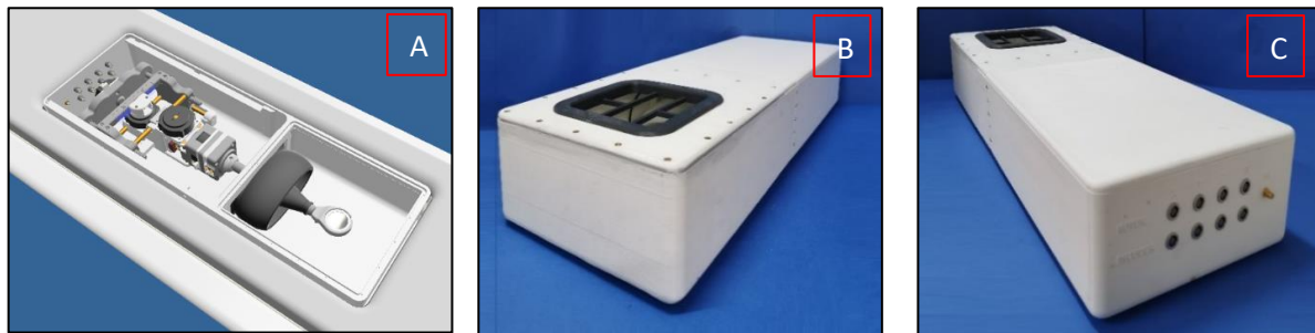
Figure 3: (A) CAD drawing of the 4DOF robotic device version 2 as integrated in the MRI bed, revealing the interior mechanism, (B) Front view photo of the manufactured device, and (C) Rear view photo of the manufactured device.
