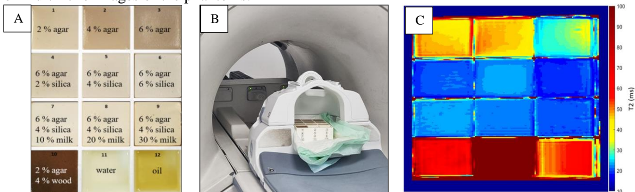
Figure 13: (A) Photo of the TMMs and the composition of additives, including the agar/wood phantom, (B) Experimental set up for T1 and T2 mapping, and (C) T2 parametric map of phantoms generated by voxel-based analysis of a series of 2D coronal MultiEcho images with different echo time values (12 - 250 ms).
