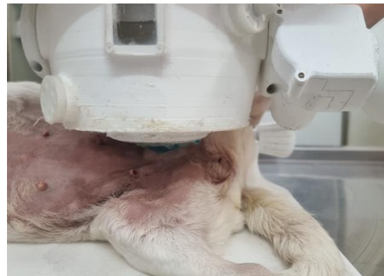
FUSVET-14 Fig. 4: Photo of coupling between the tumour and the robotic system.
