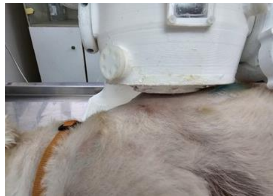
FUSVET-15 Fig. 4: Photo of coupling between the tumour and the robotic system.
