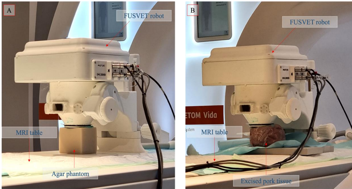
Figure 8: Experimental set-up inside the 3 T MRI scanner with the robotic system positioned on the MRI table and A) an agar-based phantom, or B) excised pork tissue, accommodated beneath the conical acoustic window of the robotic system.
