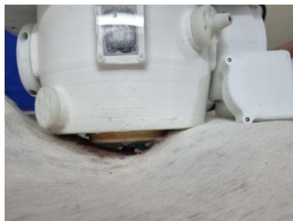
FUSVET-6 Fig. 4: Photo of coupling between the robotic system and the tumour.
