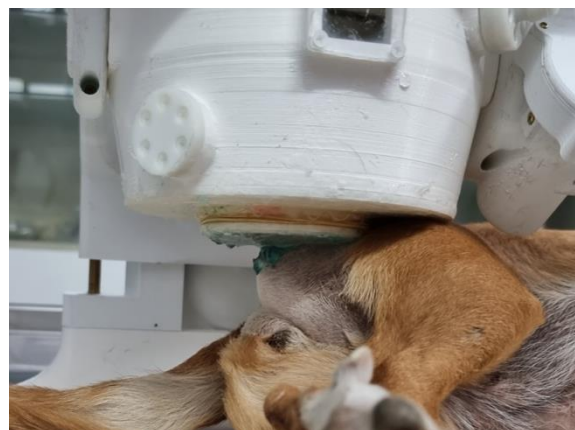
FUSVET-3 Fig. 4: Photo of coupling between the robotic system and the tumour.
