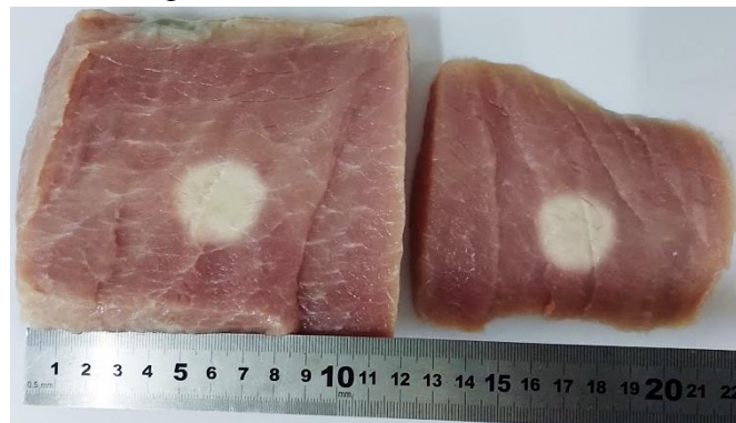
Figure 29: Overlapping lesions formed on excised pork tissue on a plane perpendicular to the beam after sonications executed at an acoustic power of 60 W for a sonication time of 20 s with motion of a 2.75 MHz transducer ( D=50 mm, ROC=65 mm) using the robotic system in a 3 \times 3 grid with a 7 mm step at a 25 mm focal depth. Slice of the tissue at 10 mm and its mirror (from right to left).
