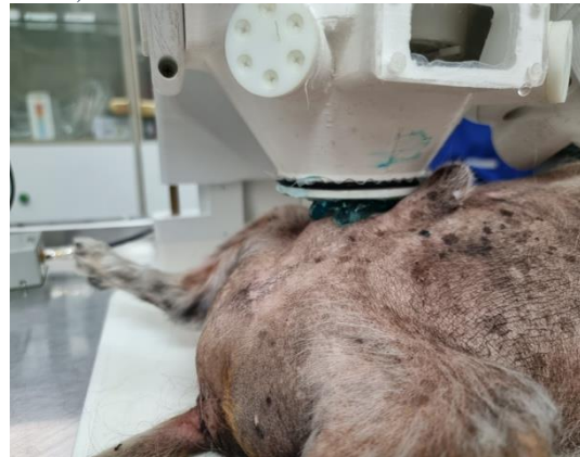
FUSVET-1 Fig. 4: Photo of coupling between the robotic system and the tumour.
