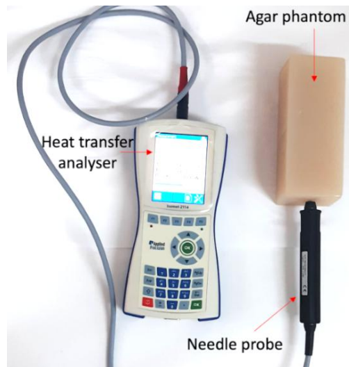
Figure 4: The experimental set-up used to measure the thermal properties of each agar-based phantom.
