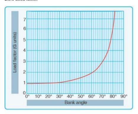
Turns—the load factor increases at a terrific rate after a bank has reached 45° or 50°. The load factor for any aircraft in a coordinated level turn at 60° bank is 2 Gs. The load factor in an 80° bank is 5.76 Gs. The wing must produce lift equal to these load factors if altitude is to be maintained.
