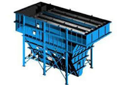
A Lamella Clarifier is a compact, inclined plate settler designed for effective removal of suspended solids from water and wastewater. It operates on the principle of gravity settling, where the inclined plates increase the effective settling area, allowing faster and more efficient clarification in a smaller footprint compared to traditional settlers. It is widely used in primary and tertiary treatment stages in various industrial processes.
