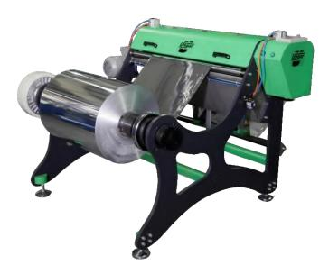
The Decoiler Unit uses a precise motor to adjust the exact speed of aluminium foil entering to press. The height of the feeding system is manual adjustable to ensure the right entrance height to the aluminium foil for the tool currently used on the press. We also provide additional **Embossing Unit** with the Decoiler system according to customer's order.
