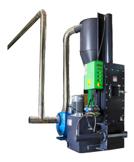
Our own manufactured ALCOMAX SBD100 Series Automatic Aluminium Scrap Collector and Scrap press machine gives our customers a good hassle free experience of complete automation and minimum manual intervention. The ALCOMAX SBD100 Series Automatic Aluminium Scrap Collector and Scrap press machine automatically convey the aluminium scrap coming out from your production line, into a collecting bin where it will be compressed into small blocks for convenient handling.
