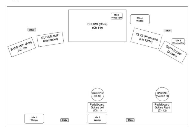
230v outlets are used for amps (back) and pedalboards (front-stage)
