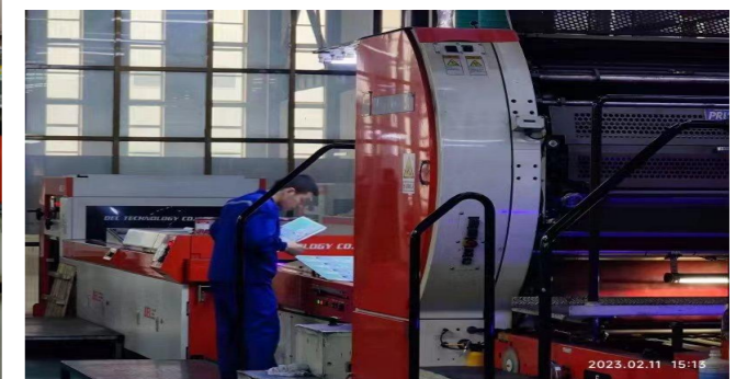
▶ 显影机 Plate processor
