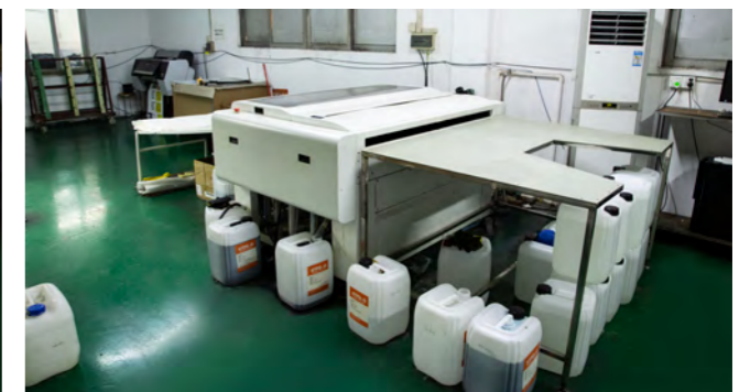
▶ 显影机 Plate processor
