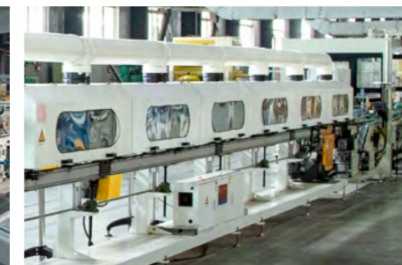
罐身外补涂电磁烘干机 Welding seam coating drying oven
