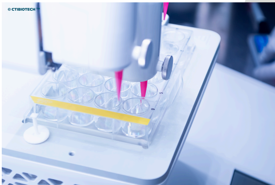
Figure 3: Automated 3D bioprinting of pancreatic microtumors in a standardized 24-well plate format for drug testing.
